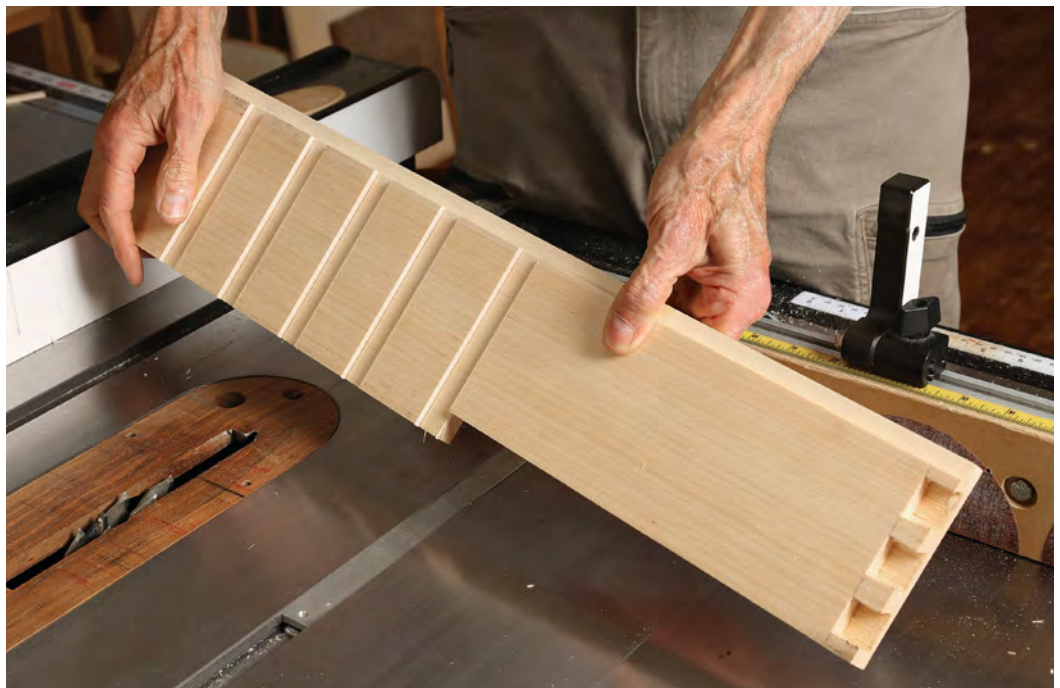
Dadoes galore. With the dado stack in the table saw use a miter gauge to cut five dadoes in each side for the horizontal dividers. Cut straight through the front of the sides; you'll cover the front of the dadoes later.
