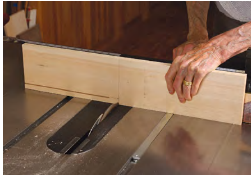
Notch it off. The notches at the top of the sides house the vertical face frames that flank the door. Create the notch with two cuts on the table saw, one ripcut and one crosscut.
