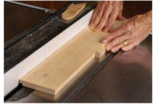
Rabbet for the back. Two more ripcuts on the table saw yield the rabbets in the sides that the back will be set into.
