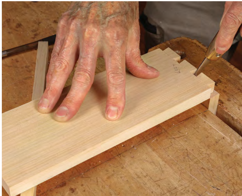
Half-blind dovetails. Connect the sides to the top and bottom with half-blind dovetails. Becksvoort cuts tails first on the top and bottom, and then transfers that pattern to the sides and cuts the pins.
