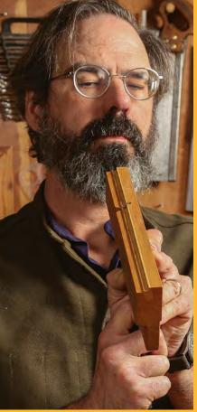
Site the iron against the sole. If the iron and sole don't match exactly you can use an aggressive abrasive on the bevel to correct the shape.
