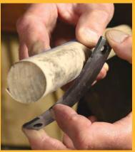
**Rock and roll.** Rock the flat side of the blade along the stone, and move your way up the grits. Remove the burr on the bevel using a dowel wrapped with fine sandpaper or diamond lapping film.
