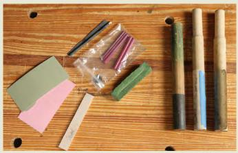
A new way to use abrasives. To reach into tight curves and rounds, use dowels in different sizes. You can wrap wooden dowels with diamond lapping film or sandpaper, or buy a pack of dowel-shaped sharpening stones in different diameters.
