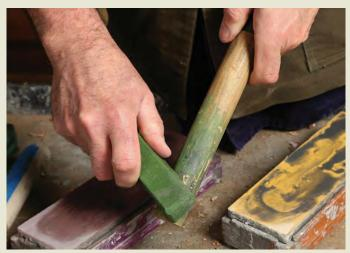
**Honing compound.** Charge a dowel with honing compound by simply rubbing the compound onto the dowel.
