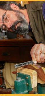
A little relief. You can speed things along a bit if you relieve some material behind the cutting edge on the flat side of the the blade using a die grinder.
