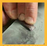
**Polish the back.** Polishing the flat back of a molding plane regularly keeps it sharp for a long time.
