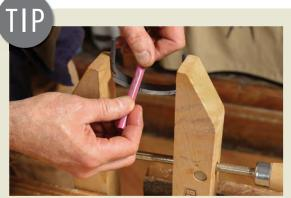
**Hand screws are an extra set of hands.** Sometimes a blade, like this travisher blade from Crown Tools, is difficult to hold for sharpening. With the blade held in a hand screw in your bench vise, you can abrade the bevel
