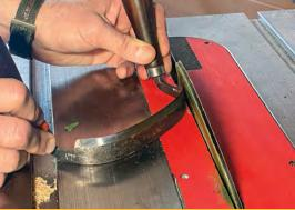
A table saw alternative. A metal plate designed to convert a table saw to a disc sander can be used to sharpen odd-shaped tools. One face has 200-grit sandpaper for grinding. The other face has MDF paper for polishing. Tilt the plate to match the tool's bevel. Charge the MDF with polishing compound. Turn on the saw and gently touch the blade to the spinning wheel.
