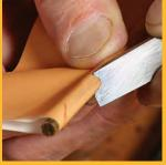
**Strop the bevel with dowels.** Schwarz either uses sharpening stone dowels or wooden dowels wrapped with sandpaper to strop the bevel. Match the diameter of dowel to the curve you're working.
