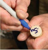
**Sanding dowels.** Adhere diamond lapping film to a sanded dowel and mark the grit on the end.
