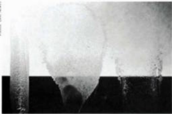
Tests on clean glass show that plain tung oil (left) dries to a badly wrinkled, opaque film. Tungseed oil (center) dries to an opaque film with tiny wrinkles. Polymerized tung oil (right) dries to a fairly glossy, transparent film.
