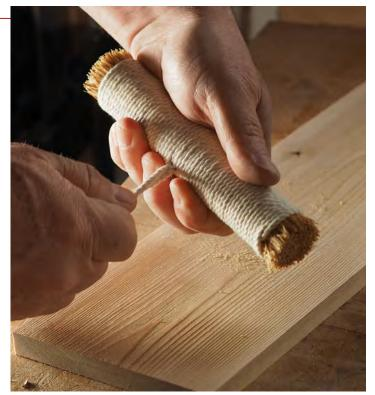
**Bound with longevity in mind.** As the uzukuri bristles wear and shorten, a pull on the binding string will expose more bristle length. A very simple but clever wrapping design allows you to pull either of the two pieces of string to expose bristles on their respective ends of the brush.
