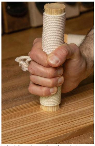
Work in shellac wax. As you near the end of your work with the brushes, rub a bar of wax along the workpiece. Then use the coarse uzukuri to work the wax into the grain while at the same time polishing and continuing to remove wood. The wax acts as a lubricant, helping to expedite the abrading process, too. Repeat these two simple steps at least a couple of times before progressing to the finer grades of uzukuri, if required.
