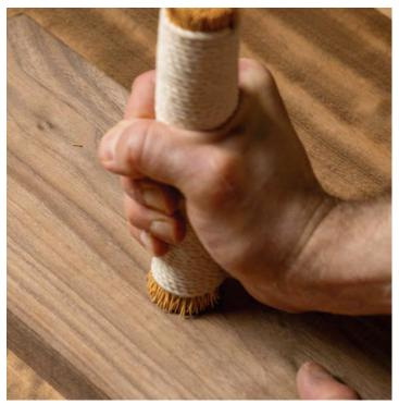
**Using the uzukuri is easy.** Hold the brush upright with one end firmly flat on the wood surface. Because the brush is bound tightly, which adds rigidity, but can flex and give when working the surface, it is best to grip it firmly and as near the working end as comfortable without touching your hand to the wood.
