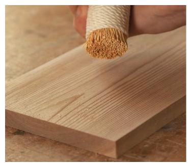
Roughing it up. The most important brush is the rough one. In most cases, it takes care of at least 90% of the work and may be the only brush you use. As you work the surface of softwoods with the rough brush, you will see dust forming and collecting at the end of each stroke. That is the soft wood being brushed out of the surface. This gives you instant feedback. On hardwoods, very little dust forms so it is best to work with raking light to monitor your progress.
