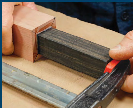
Align and clamp. Align the corners of the foot with the crossed lines on the leg, and clamp the joint with a single bar clamp. Position the clamp carefully so the foot goes on straight.
