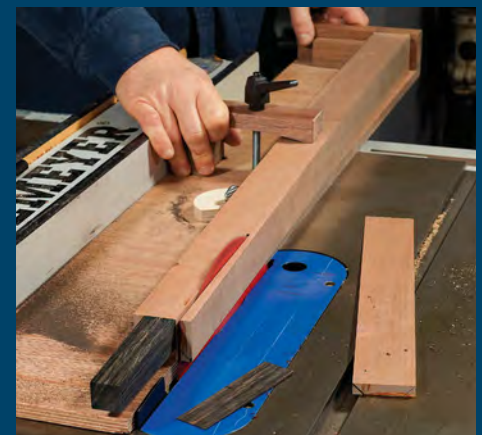
Taper the leg and foot. Use a sled-type jig and remember to reposition the stops after the second taper is cut.
