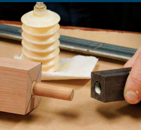
Spread glue and assemble. Squirt some glue into the holes, spread it with a small stick, and spread some on the end grain and dowel as well.
