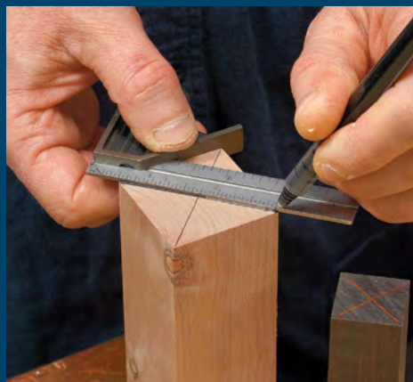
Mark centers. The foot blank is smaller than the leg blank, saving some of the expensive wood used for some feet. Connect corners to mark centers.
