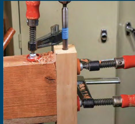
Drill for dowels. Move the drill-press table to one side and clamp on a square block as shown to hold the parts vertically. Drill at least 1\frac{1}{2} in. into each part.
