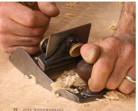
tightening is needed, or if the cut favors one side, reset the blade. Cutting properly, the tool should make a shaving almost as wide as the blade.
