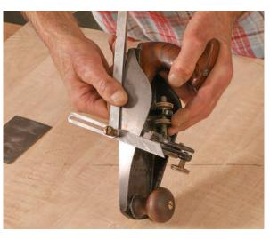
**Insertion.** As with the No. 80, you insert the blade with the bevel facing you and press it firmly to a flat surface. Then tighten the blade with the knurled knob.
