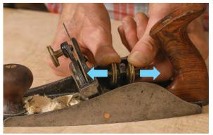
**Tilt the blade for a heavier shaving.** Unlike the No. 80, whose thinner blade can be flexed with the center thumbscrew to take a heavier cut, the No. 112 and No. 12 are adjusted by changing the blade angle. To take a more aggressive shaving, turn the twin knobs to tilt the blade farther forward. For a lighter cut, tilt the blade backward.
