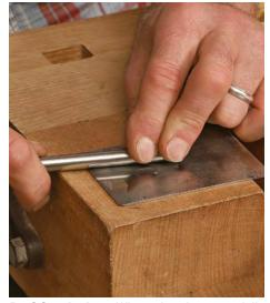
**Reviving the burr.** When a burr becomes dull, press the burnishing tool several times along the back of the blade with moderate pressure to draw out the first burr. Then turn a new burr.
