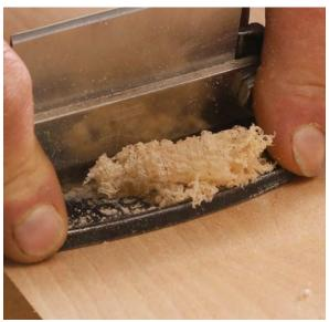
Tightened up and making shavings. With the blade adjusted properly, fully tighten the blade-holder screws to lock it in place.
