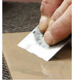
**Polish the bevel.** Holding the blade so its bevel is flat on the sharpening stone, hone the bevel with a few strokes.
