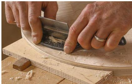
**A friend for fine work.** Just like a card scraper can, a cabinet scraper will work delicate and difficult solid and veneered surfaces to a beautiful finish regardless of grain direction. Working this circular veneered tabletop, Coleman scrapes from the center out to the edge; because of the No. 80's short sole, scraping in from the edge isn't advisable.
