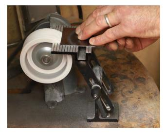
Then grind the bevel. Unlike a card scraper, whose edges are square to its faces, the cabinet scraper blade gets a 45° bevel along its cutting edge. The bevel can be straight across or slightly cambered. And you can file the bevel instead of grinding it if you choose.
