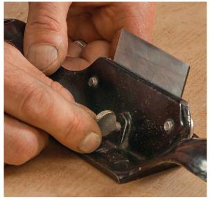
The bevel can be ground straight across the edge or with a slight camber. In use the blade wears most in the center and a camber helps mitigate this. To avoid cutting myself on the exposed top edge while using the tool, I slightly round the corners of the blade at the grinder. For fine work, I hone the bevel to a mirror polish before turning a burr.
