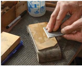
Flatten the back first. Just as he would with a plane blade, Coleman hones the flat side of the scraper blade to obtain a mirror finish behind the bevel.
