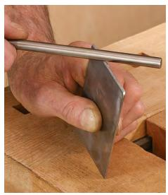
**The burr stroke.** To create the burr, draw the burnisher across the top of the bevel applying light pressure and holding the tool at a bit less than 90° to the face of the blade.
