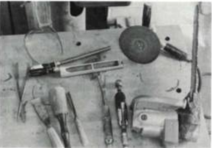
Chain saw, Surforms, pneumatic gouge and ball mill, gouges, rifflers and sanding disc are used for shaping. Then the top transition pieces are assembled and aligned.
