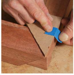
of cardboard over the apron's miters. The cardboard, cut to match the shape of the mitered wing of the apron, ensures the clamping cauls focus their pressure only there. The cardboard's necessary in case the wing sits too low in the leg recess, allowing the leg to interfere with the cauls.
