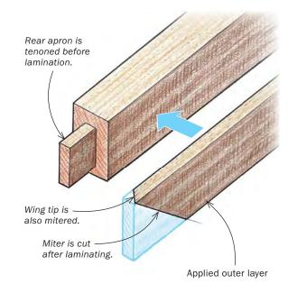
Mark the miter % in. long. Then sneak up on the cut. Because of this joint's complex geometry, don't try to lay it out perfectly. Rather, use a pencil mark to get you in the ballpark before working up to the final fit at the table saw.
