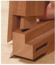
Assemble the three-way miters after dryfitting with clamps. During the final testing of the joint, apply clamping pressure to simulate final assembly.
