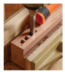
Mortise the leg. These mortises accept the tenons on the apron. Be mindful of your reference faces as you flip the workpiece for mortising.
