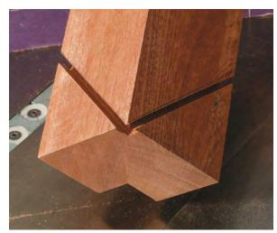
The miters should meet at the corner. The meeting point of the angled shoulders should be at the corner of the leg. If it's slightly below, that's OK, because you'll trim the apron's mitered wing to fill the space.
