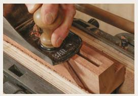
If the tenons seat but the miter remains open, carefully plane the leg's mortise face. This will make the mortise shallower, so be sure the tenon does not bottom out. Shorten it if necessary.
