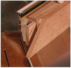
Mark the wing tip, then sneak up on the cut. In order for both aprons to seat at the same time so the full joint can come together, you need to cut a second miter at the outside tip of the apron. This miter runs from the outside tip to the inside face. When sawing it, Coleman lines up the outside tip of the apron's miter with the sawblade.
