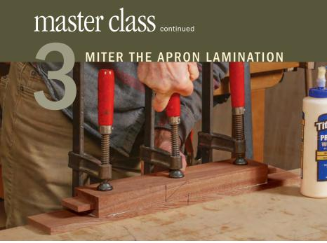
**Glue the apron's thinner outer layer to the tenoned rear board.** The applied show face is overlong and slightly wide here, so Coleman doesn't have to fret about locating it perfectly on the tenoned piece. He flushes the edges of the applied face to the rear piece after the glue dries.
