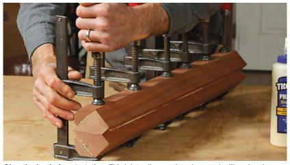
**Glue the leg halves together.** This joint relies on glue alone, so be liberal and use plenty of clamps. After the glue sets, pry off the cauls and clean up the surfaces. Keep the faces straight and square for the joinery. Cut the ends square and to length.
