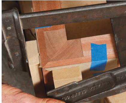
Glue up all at once. The narrow cauls direct pressure right over the apron's miter, keeping it tight to the leg recess. Coleman uses heavy-body epoxy from Epo-Tek because of its 30-minute open time, letting him seat and check all four corners. Plus, the epoxy's paste consistency keeps it from running.
