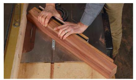
**Cut the second shoulder after adjusting the miter gauge to its other 45° setting.** Having a reliable miter gauge with positive stops at 45° will make these cuts (and subsequent ones) much more manageable. Make this second shoulder cut with the fence at the same setting.
