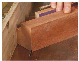
This long miter can be tricky to clamp, so I use shaped cauls glued temporarily to the leg halves. The cauls' shape matters. I take the triangular cutoffs from sawing the long miters and trim off their apexes, yielding a shape with two parallel faces and 45° edges. I glue the cauls to the leg halves with a paper joint, placing the clamps on the flattened apexes. When that glue dries, I glue up the two halves of the leg, using the 45° edges of the cauls to clamp across the miter.
