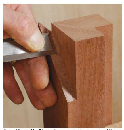
**Undercut the shoulder.** This precautionary measure ensures there are no high spots of end grain that will prevent the finished joint from closing.
