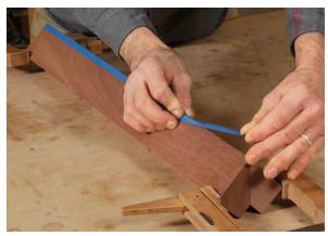
**Tape the miter.** Coleman runs a strip of tape along the whole joint. The tape keeps the leg halves aligned, first with the miter dry, as he attaches clamping cauls with a paper joint; and later when he glues and clamps the long miter.
