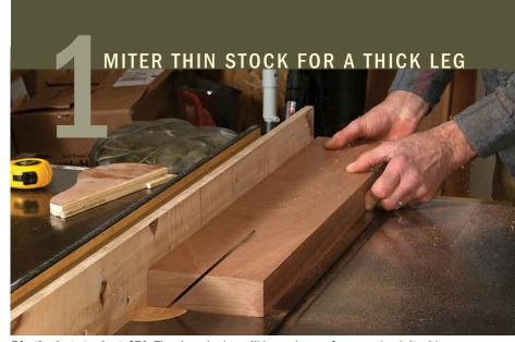
**Rip the leg stock at 45°.** The ripped edge will be a glue surface, so check it with a miter square and straightedge. Coleman uses offcuts from these rips to make clamping cauls.
