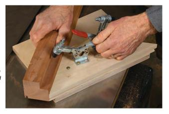
Press the jig tight to a tall fence and the saw table to rip the cheeks. The jig's tall fence needs an auxiliary tall fence on the table saw for safety and accuracy. For cuts on both sides of the ramp, Coleman pushes the entire jig through the cut.
