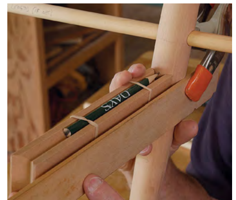
Mark the drilling location too. A pencil secured in a long V-block lets Durfee mark exactly where to drill. A straight stick of wood clamped to the leg ensures the block sits in the same plane as the leg.
