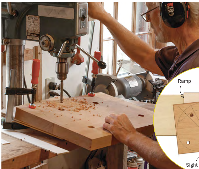
Start with the two center spindles. These are stopped mortises. Set the point of the drill into the spot for the spindle hole, then rotate the seat blank so the sight line is straight toward you.
