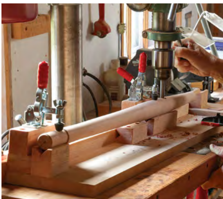
Support the leg while drilling. After tilting the drill press table to the correct angle, Durfee sets up a jig to stabilize the leg. Its long platform has V-blocks to cradle the workpiece, including one right under the drilling locations. Its toggle clamps ensure the leg stays put, too.
