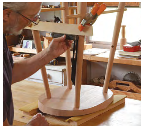
Dowels align legs for determining angle for side stretchers' holes. To make sure the legs are oriented correctly, insert a dowel through the stretcher holes you just drilled. Dowels also help when getting the shoulder-to-shoulder dimensions for the stretchers.
