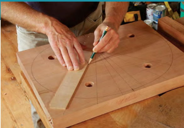
Determine the spindle sight lines. On the top of the blank, connect the spindle locations to their convergence point along the centerline. You'll sight down these lines when drilling mortises for the spindles.
