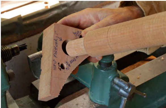
Test the turned tenons. While turning the legs and tenons, Durfee frequently checks the latter against a test hole bored with the same bit he used to drill the leg holes in the seat.
