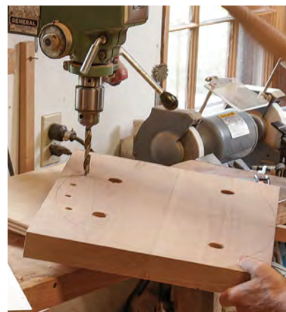
The outer spindles need a shim. The four remaining spindles need a touch higher ramp angle than the others to line up correctly. To adjust them, Durfee shims up the seat \frac{3}{32} in. before drilling.
