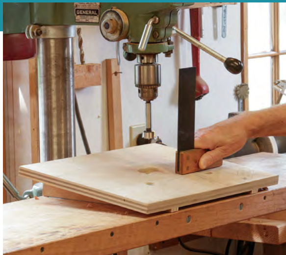
Reset the drill-press table but leave the ramp. The spindles tilt back, but they don't splay. So bring the table back to square without moving the ramp.
