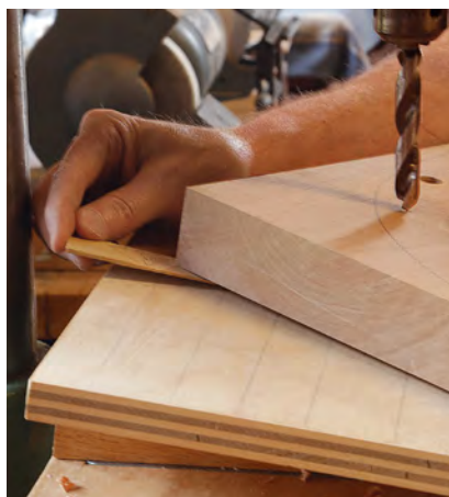
The outer spindles need a shim. The four remaining spindles need a touch higher ramp angle than the others to line up correctly. To adjust them, Durfee shims up the seat \frac{3}{32} in. before drilling.
