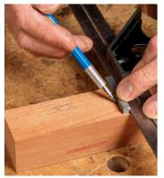
Lay out the top and bottom of the mortise. Line up the top edge of an apron with the top of the test leg and set your square on the bottom edge of the apron. Butt a spacer to the square, and strike a line to represent the bottom of the mortise. Use the square to mark the top of the mortise if it's a straight-up mortise or the bottom of the haunch if it's haunched.
