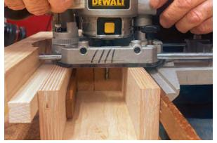
using. They must be the same diameter as the original rods. Drill holes for them in the keeper fence spaced to match your router, then epoxy them into the keeper fence.
