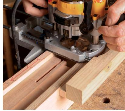
**Cutting the haunch is simple.** After cutting the main mortise, you can cut the haunch in one or two passes. Depending on which mortise you are cutting, you'll start from the end of the leg and cut toward the main mortise, or start in the main mortise and cut to the end of the leg.
