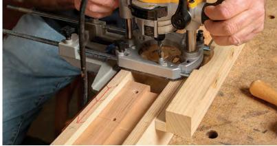
**Plunge, plunge, and back and forth.** Van Dyke's preferred cutting method is to make full-depth plunge cuts at the start and end of the mortise, and then make progressively deeper passes the length of the mortise until he reaches full depth. His pro tip: Don't change the router depth at the end of each pass. Instead, first slide the router back to the beginning. This pass will clear any chips without cutting wood.
