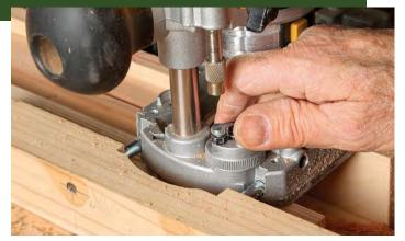
**Turret stop sets depth.** Once you cut the full mortise, you can focus on the haunch. The only thing you need to change on the router is the depth of cut.
