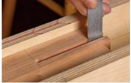
Check your depths. Before you remove the leg, use a metal ruler inside the mortise to double check the depth of the main mortise and the haunch.
