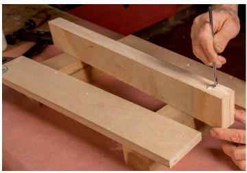
**Ready to glue.** Spread glue on the edges of the bottom piece (two ganged pieces of <sup>3</sup>/<sub>4</sub>-in. plywood).
