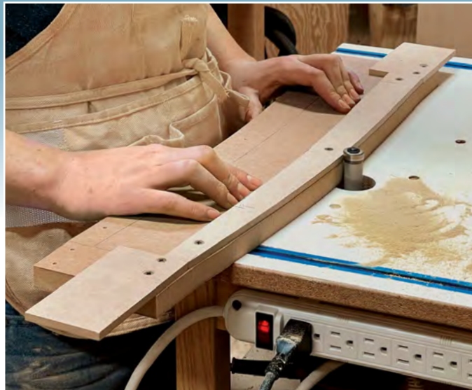
Shape the router jig. Screw the leg template to the jig's base and cut the curve using a pattern-routing bit. On the convex side, add blocks to the ends of the template to create smooth entry and exit areas for the router bearing. Before removing the template from the jig, trace its back edge and ends, to show where stop blocks need to go.
