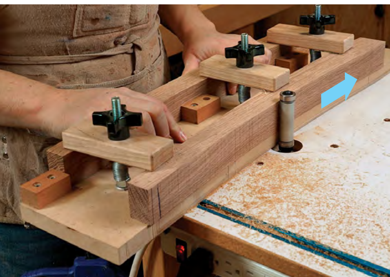
Route the concave side first. Use a long flush-trimming bit. Line up the leg with the pencil mark on the jig, let the waste part of the leg overhang the edge, and clamp it in place (you'll need another leg in the jig to make the clamp blocks work). Move the jig right to left to rout.
