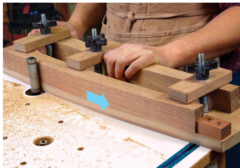
Route the convex edge second. The concave edge is placed against stop blocks on this side of the jig, as is the end of the leg. Move the jig from right to left again.
