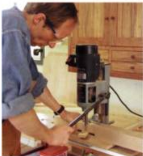
Notch it. After cutting the mortises for the rail tenons, the author uses a hollow-chisel mortiser to notch the posts where they accept the corners of the cabinet top and cabinet bottom.
