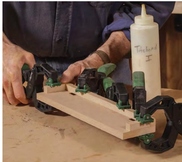
**Add the fence and end stops.** Glue these flush to the base's perimeter to ensure they're square and spaced symmetrically.
