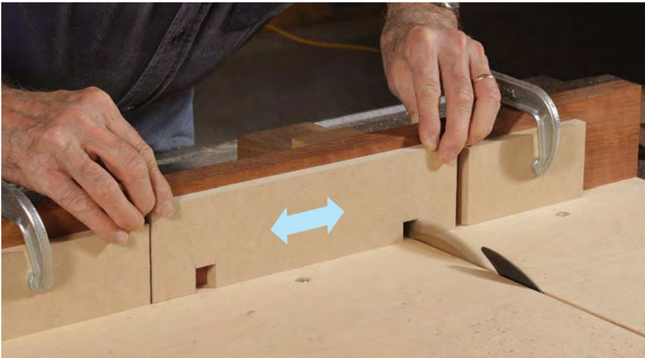
**Clamp a pair of stops to a sled to notch the jig base.** The stops should be set to yield a notch the width of the hinge leaf. When setting the blade height, add the desired width of the hinge mortise to the width of the jig's fence. Slowly advance the sled while sliding the base side to side to cut the notch. Check the fit (right), and then flip the base to cut the second notch.
