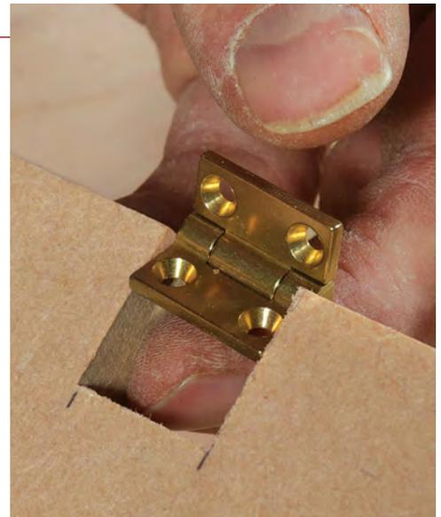
**Test the notch's width against the hinge.** It's best to start with the stops a little too close together, then move one farther away as you sneak up on the correct width.
