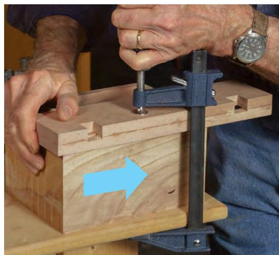
**Slide the jig tight to the other side for the other hinge.** Because the jig's notches are the same size and the same distance from the base's ends, setting up for the box's other hinge is a simple matter of sliding the jig.
