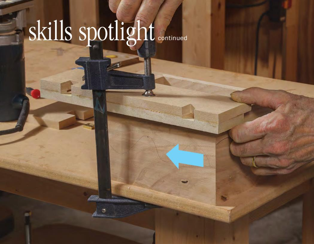
**Snug the jig to a corner of the box and clamp everything down.** Double-check that the fence and end stop are tight to the box. Clamping to the workbench ensures nothing will move while you are routing.
