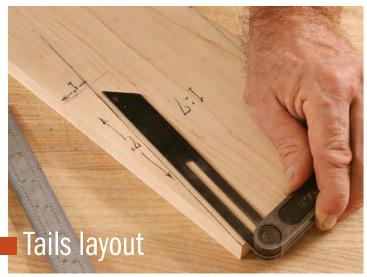
Simple setting. Strazza likes a 1:7 ratio for the angle of houndstooth dovetails, and a quick drawing on a scrap guides the setup of his sliding bevel.
