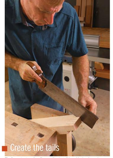
**The important angles.** Strazza tilts the tail board in the vise so he can monitor the layout lines on the end and the face; then he cuts the dovetail angles with a tenon saw.
