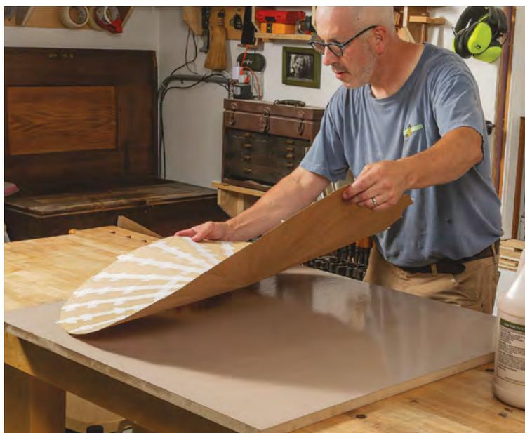
**Glue the veneer to the substrate.** Eaton uses a square of  $\frac{3}{4}$ -in. MDF a couple inches larger than the diameter of the veneer circle. He applies glue evenly to the substrate only, not the veneer.
