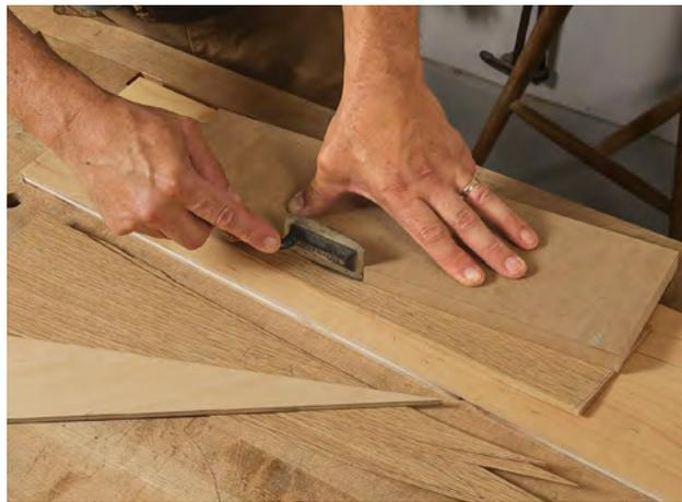
**Saw through the stack using a straightedge and backer board.** The straightedge is a piece of MDF that Eaton holds in place by hand. The backer board protects both his bench and the bottom face of the veneer.
