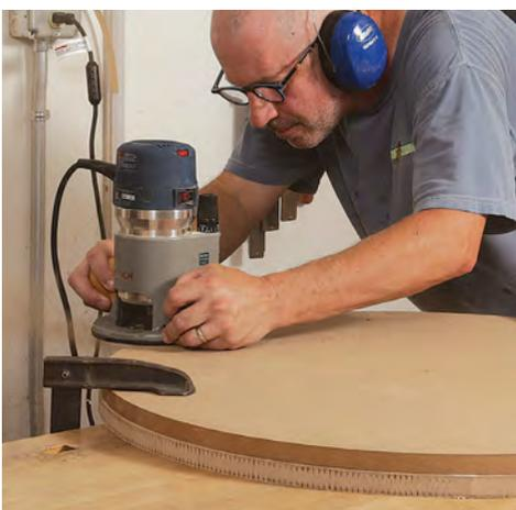
**Pattern-route the top to shape.** To keep the piece secure, Eaton uses beefy clamps and hangs only a bit of the top off the bench. This means he can rout only a little before having to rotate the top, but it keeps the setup vibration-free.
