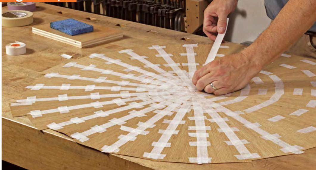
**Apply veneer tape to the front.** Stretch multiple short pieces across each joint and then one long piece along its length. To minimize denting, don't stack more than two or three strips of tape. Shorten or stagger the tape toward the center. Finally, remove the masking tape from the back.
