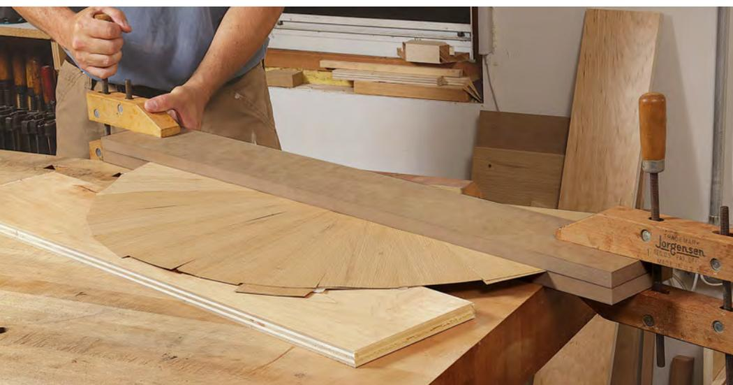
**Clamp the halves together, then joint them simultaneously.** Clamp the halves between strips of MDF to keep them rigid. You may need to plane from both ends because the grain reverses at the center.
