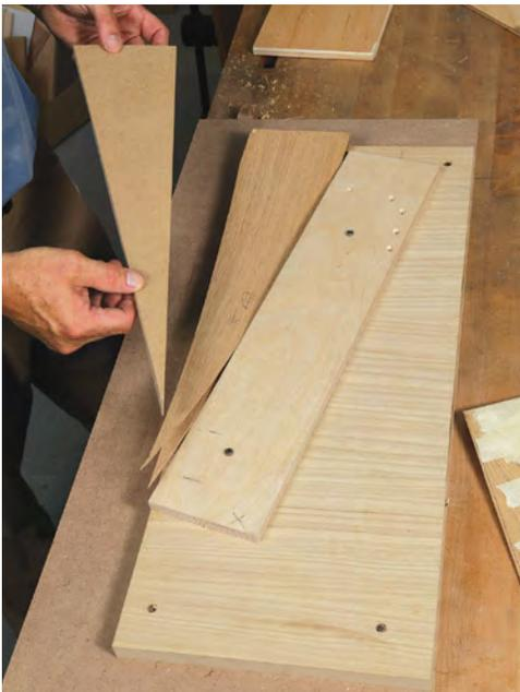
**Joint the edges using a shooting board with an angled fence.** This quick-to-make jig holds the segments at the appropriate angle for truing up their edges so they're glue-ready later. To hold the segments flat to the jig, Eaton tops them with a wedge of  $\frac{3}{4}$ -in. MDF.
