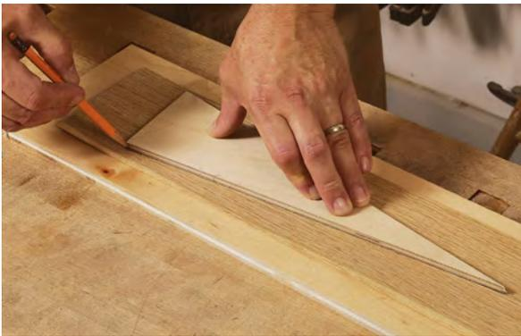
**Trace the segment pattern onto a short stack of veneer.** Eaton makes a template of the pattern, a wedge cut to the correct angle. He uses it for fast, repetitive marking on three to four pieces of veneer at a time.
