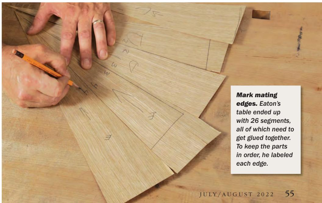
**Mark mating edges.** Eaton's table ended up with 26 segments, all of which need to get glued together. To keep the parts in order, he labeled each edge.
