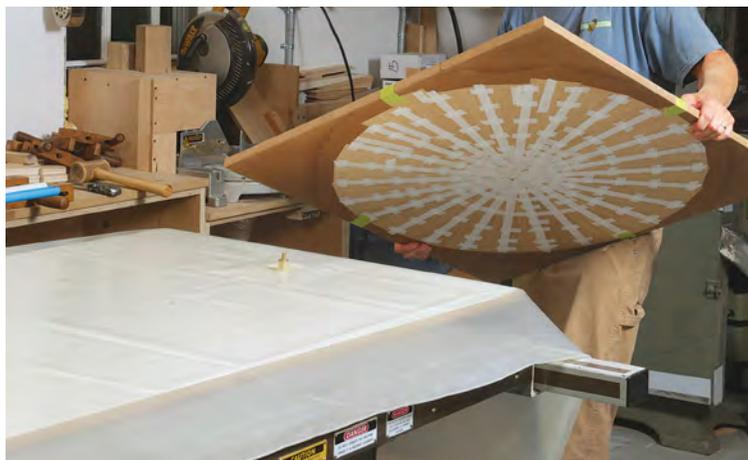
**Painter's tape keeps the veneer from slipping in the vacuum press.** The tape holds the layers in place as you slide the panel into the press and also secures the package as the press tightens.
