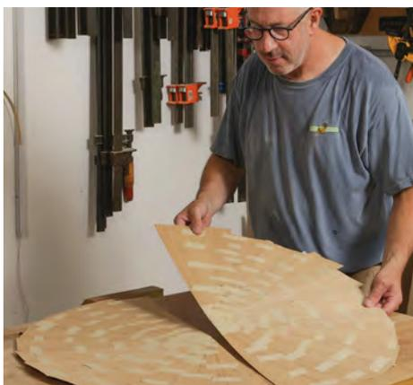
**Tape the halves in back to hold the circle together.** Now jointed, the halves are ready for masking tape on their back faces. As before, pull the tape taut across the seam.
