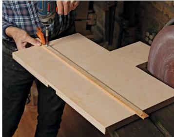
**Add a runner.** To square up the base to the disc, you'll need to make a runner to fit the slot on the table of your sander. Make it a few inches longer than the base for now. Screw one side of the runner to the base.
