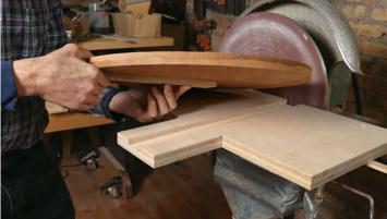
**Get centered.** After bandsawing close to the line of the final shape, place the sharpened brad into the workpiece at the circle's center point. Then flip that assembly so the workpiece is on top, and fit the bar into the baseplate.
