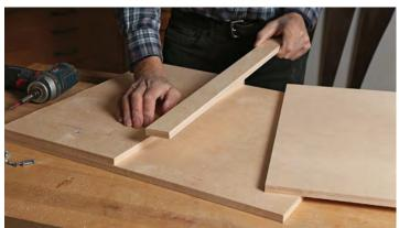
**A plywood stack.** The bottom layer of plywood is one sheet. Line up the first partial sheet on top of that. Glue and screw it to the bottom. Keep the glue away from the center slot so you don't glue your spacer in place.
