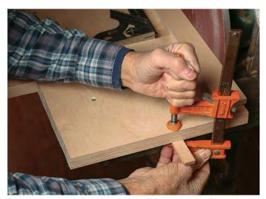
**Secure the runner.** Once square and still in place at the disc sander, carefully clamp the unsecured end of the runner to the base. Now you can take the base off the sander and screw the clamped end to the base.
