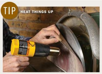
It's easy to remove the sandpaper from the disc. If it doesn't peel right off, heat it with a heat gun or hair dryer until the adhesive melts and the paper peels easily.
