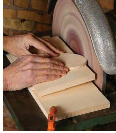
**Bevel your curves.** This jig allows you to present straight or curved edges to the sanding disc at an angle. Clamp the jig to the sander table, and work to your line.
