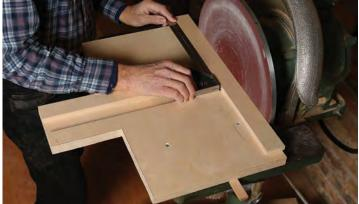
**Square the base to the disc.** Insert the base into the slot, with only one side of the runner secured. Then adjust the opposite side until the slot is perfectly square to the disc face.
