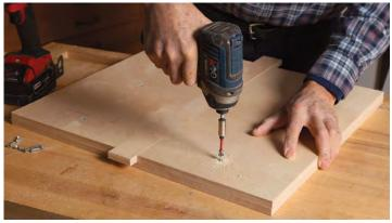
**Create a slot.** Position a spacer up against the first sheet of plywood on the top layer, and glue and screw the other piece of plywood directly against the spacer.
