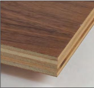
Veneer-core plywood is an extremely useful material because it is easily available, very sturdy, structural, and extremely stable if made well. When clients want wood faces for casework, opt for the strength and screw-holding power of plywood for the boxes. You also can use 1-in. veneer core for shelves as it is stronger than MDF, which tends to sag.
