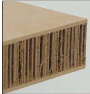
Think of these products as a futuristic model for what plywoods might become. The core of this sci-fi sheet good is made of materials including fiber, cardboard, foam, and PC2 polycarbonate plastic. This substrate will keep any panel rigid, flat, and super-light. The product's core, in a grid resembling a bees' honeycomb, is sandwiched between thin skins of HDF or MDF; the combination creates a strong,
