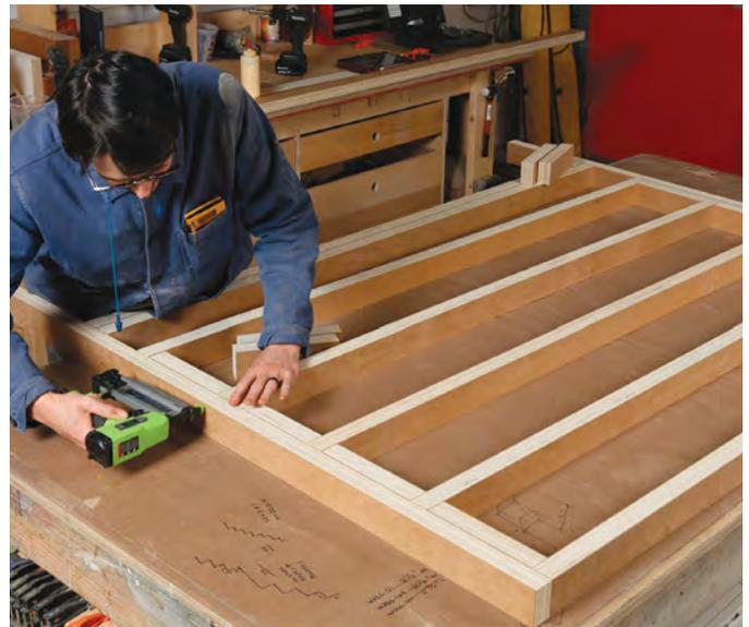
**Your framing friend.** Garnica is an ideal material for framing. It is flat, strong, light, and easier to rip into dimensional parts than wonky 2x material. Rowan frequently uses it in places such as inside a kitchen island, creating a chase for the electrical and plumbing. Or here, as the infrastructure holding a built-in bed together.
