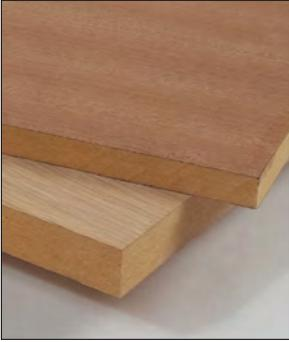
Because it's an engineered material, MDF doesn't have grain patterns, which gives it a smooth finish ideal for paint or veneer, and a consistent, stable thickness. An MDF core panel with a pre-applied veneer is the absolute best product for cabinet doors and drawers. Completely void-free, it makes for a very flat surface, and the fibrous core won't move while it's being cut or after installation.
