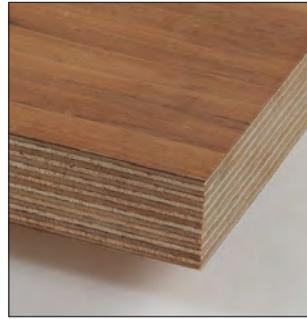
When you're after that exposed edge look, ApplePly is another great option. Like its European multi-ply competition, it has a lot more ply layers than typical plywood (both have 13 plies per 3/4 in.), making for a very good aesthetic. Appleply is manufactured in the United States using a mix of aspen and maple trees, setting it apart from the birch and poplar hardwood cores used in Baltic birch and Russian birch.
