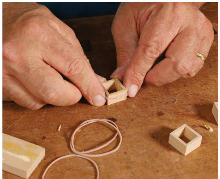
Elasticity. A doubled-up rubber band provides clamping pressure as the square cures.
