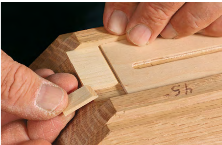
Back into the miter jig. After resetting the jig's stop, Stevens presses the mitered end of the strips against it.
