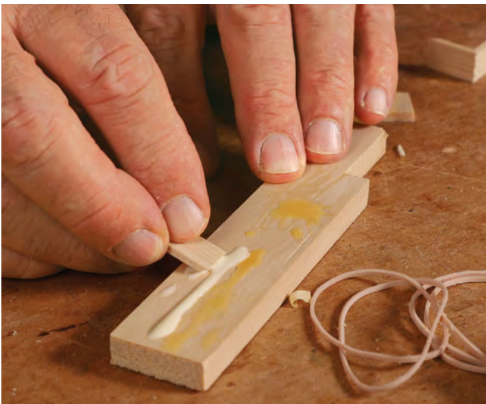
A little dab of glue. Working on a flat surface and applying a smear of white glue, Stevens presses the squares together.
