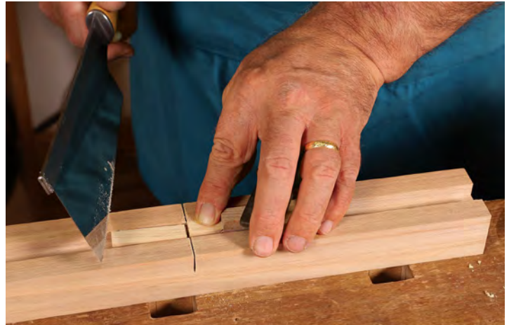
Saw to rough length. The strips are then stacked in a miter box, with their miters against a stop, and cut to rough length.
