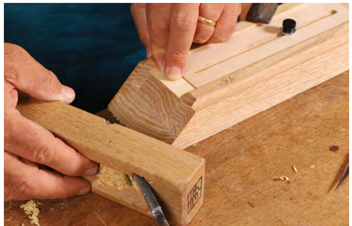
Miter number 2. A few strokes of the plane create a second miter, finishing all four pieces.
