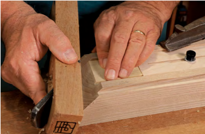
Make the first miters. With a handplane and a miter jig, Stevens cuts miters on four strips at once.
