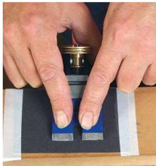
After marking the top of the frog with a felt-tip pen, grind it on 240-grit wet-or-dry paper stuck to a smooth, flat surface. The center felt-tip lines should be removed.
