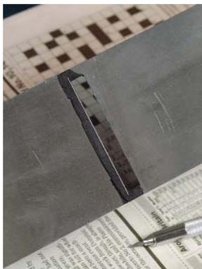
To prepare the throat for filing, mark the sole with a black felt-tip pen, then scribe a line as close to the mouth as possible (above). Then clamp the plane body in a vise, angling it 15° from vertical. Keep the file parallel to the top of the vise and gradually file the throat back 15° (right) until the new bevel reaches the scribe line.
