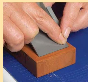
**Create a curved edge.** By concentrating pressure first on one side of the blade and then on the other, the cutting edge acquires a slightly convex profile.
