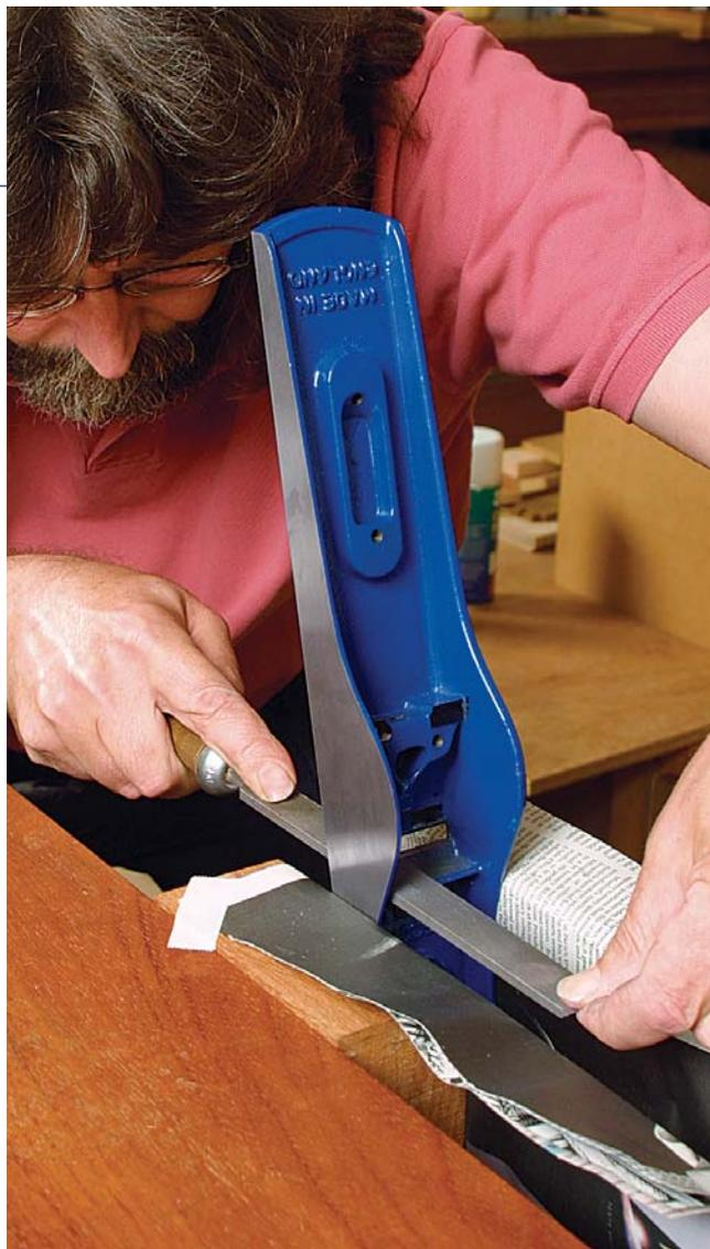
nounced hollow in the critical area on top of the frog that supports the blade just behind its bevel. This hollow can cause chatter during planing. A rough surface also may impede smooth blade adjustment. It is not necessary to remove every scratch from the top of the frog; just aim for an overall flatness.
