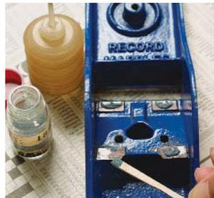
Apply a small amount of silicon-carbide powder to each contact point, add a drop of water, and then slide the frog back and forth to give the metal a smooth finish.
