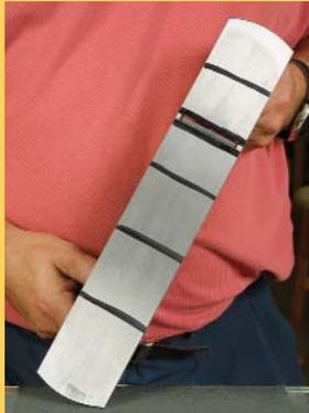
Mark the toe, both sides of the mouth, and the heel. When these four lines are sanded away at the same time, the plane is ready to use. On a flat surface such as float glass, stick down a few different grades of wet-or-dry sandpaper. With the blade installed but backed off, flatten the sole by sliding the plane over the sandpaper.
