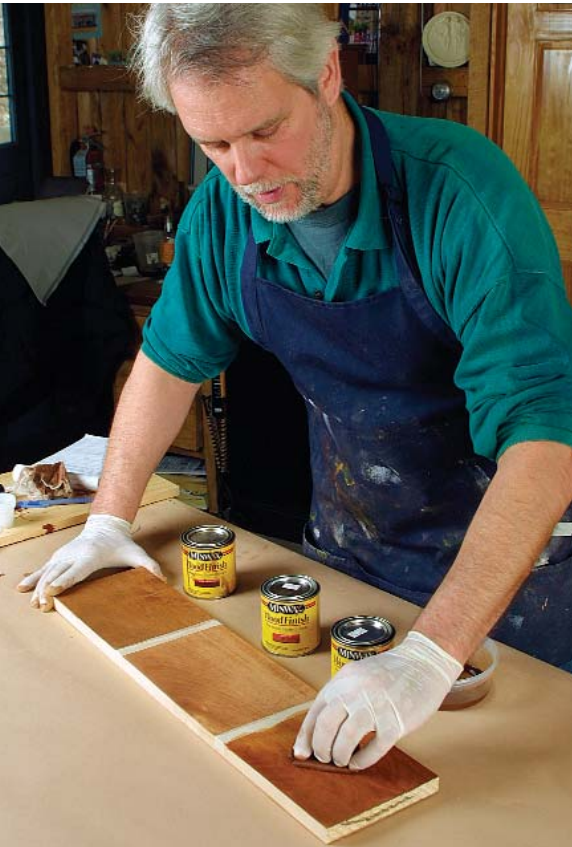
Always make a sample board. When mixing colors, it is important to test them on scrap-wood before applying them to the workpiece.
