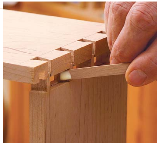
Engage the joints before adding the glue. Get all four corners started before applying the glue. Then work quickly to apply the adhesive to all mating surfaces.
