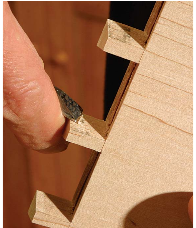
Shave off the excess with a chisel. The graphite left on the sides of the pins will tell you where you still need to remove material to get the joint to fit perfectly.
