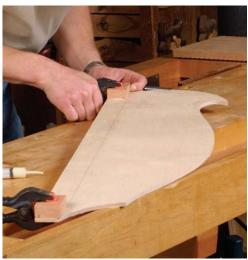
Glue scrap blocks to the template. The blocks prevent the bit from catching the corner of the workpiece and damaging it upon exit and entry.
