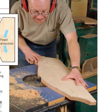
that are known as flush-trimming bits when the bearing is on the tip, and pattern or template bits when the bearing is on the shank. You need one of each type; mine are ½-in. bits with a cutter length of 1 in. When using these straight bits with templates that are exactly the size of the finished piece, there's no need to add offset for a bushing, and no worries that a bushing may be off center.
