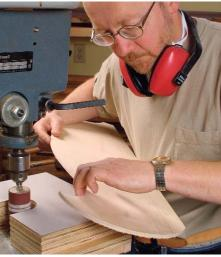
**Cut and sand the template.** After roughing out the template on the bandsaw—cutting ½ in. outside the line—smooth the template to its final shape using a belt sander (left) for flat or convex areas and a drum sander (right) for inside curves. Subtle irregularities are difficult to see, so inspect your template for dips and bumps by running your hand across its edge.
