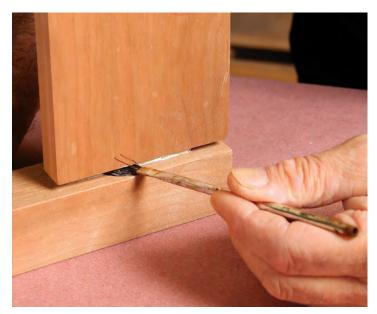
A smart glue-up strategy. Brush the glue into the mortise, and around the tenon, putting a thin coat on the end grain shoulders of the tenons. Before you seat the tenon all the way in the mortise. stop and brush out the roll of glue that forms as the tenon goes into the mortise. This will help eliminate squeeze-out.
