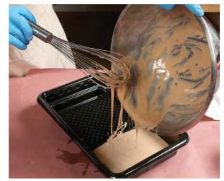
Measure and mix. Unibond, a urea formaldehyde glue, is available in a twopart system, like epoxy. Once you've measured out the powder and the liquid (1 part powder to 4 parts liquid or 1:6 for a slower dry time) mix them together. Van Dyke pours the mixture into a paint tray and rolls it onto the work. Unibond cures to a rigid, strong bond, making it a solid choice for bent laminations. Roll the glue on one side of each lamination as vou stack them.
