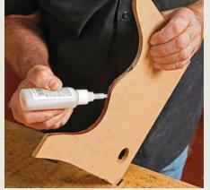
**Seal and harden.** Spreading medium thick CA glue and spraying an accelerator on MDF templates seals the edges and hardens them, allowing a single template to last through years of repeated use.
