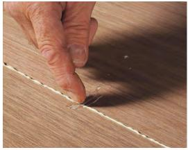
A level glue-up makes flattening easier later. Use spring clamps to hold the boards flush, testing flatness with a finger. Before adding clamps across the top, scrape off any squeezeout. This allows the glue joint to dry faster. Add the top clamps, then flip the panel and remove the glue from the bottom as well.
