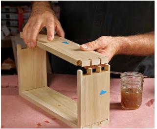
minutes) means it has a correspondingly long clamp time (the time required for the glue to set sufficiently to allow the clamps to be removed without compromising the joint), which becomes an unnecessary disadvantage when that long working time is not needed. Removing the clamps on an unstressed glue joint in less than four hours is asking for trouble. Leaving the joint in clamps overnight is safer but can be inconvenient.
