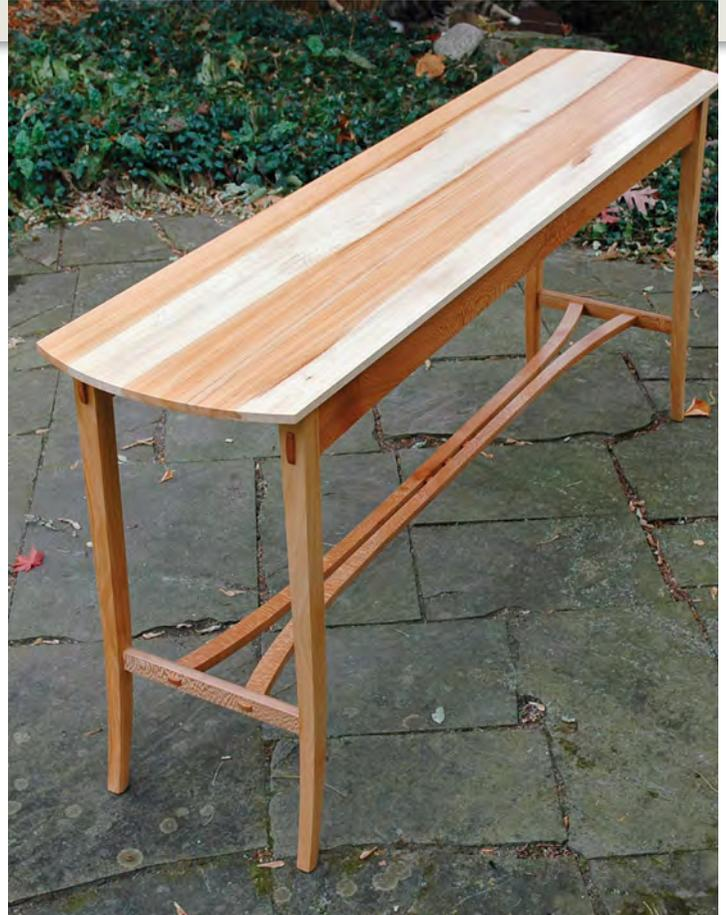
**Elevate a simple form.** The long, low, double stretchers on this quartersawn sycamore hall table curve in toward each other and connect to the side rails with through-tenons. They stabilize the structure while their curves lend the piece more intrigue and complexity, playing off the subtle curves of the legs and the ends of the table.
