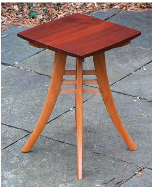
**Crisscross apple sauce.** This mahogany and birch table is a bit of a showoff. Made from wood salvaged from a 1930s dining table, the four splayed legs connect with six alternating stretchers (three between each pair of opposing legs) that cross and overlap each other in the center.
