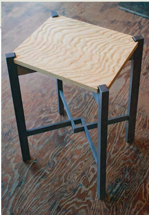
**Tenons and lap joints take over.** The lean structure of this wavy red oak and walnut table is shored up with intersecting, overlapping stretchers that lock all four legs together.
