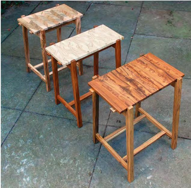
**An experiment with scraps.** These small tables made with shop scraps of maple, buckeye, and Jamaica dogwood play with the rail-to-stretcher idea. On the narrower table Gilpin uses one stretcher between the rails, but he added a second rail on the wider ones. They firm up the structure and evolve the design.
