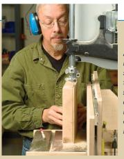
And adjusted the carriage for drift. After installing each blade, a test cut was made on a scrap block of wood to determine the angle of blade drift; then the carriage was adjusted to match the angle.
