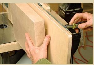
Then mounted the test blocks securely to the carriage. Each test block was screwed to the carriage before the test cuts were made.
