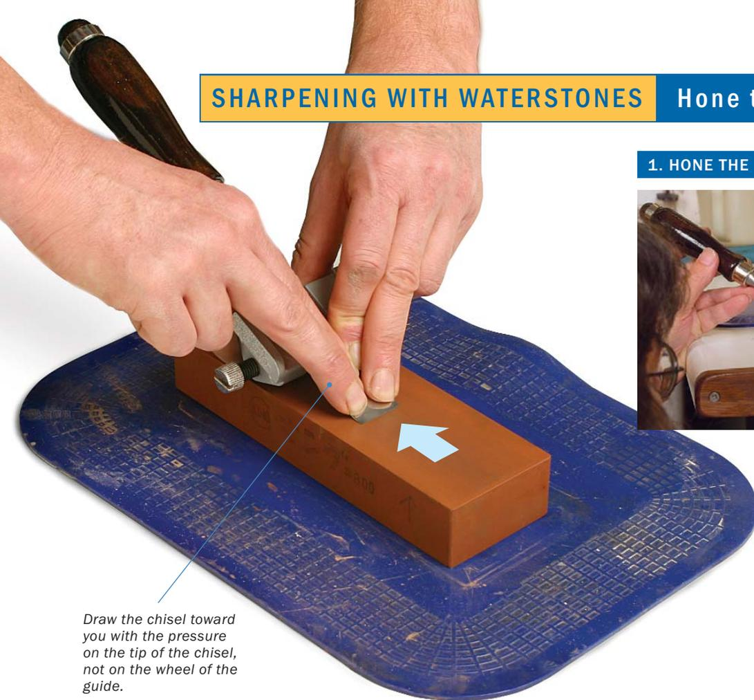
Draw the chisel toward you with the pressure on the tip of the chisel, not on the wheel of the guide.
