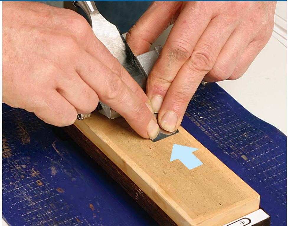
**A few light strokes.** Establishing the final cutting angle on the 8,000-grit stone requires only three or four light pulls.
