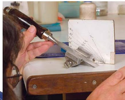
**Set the bevel angle.** With the chisel mounted in a honing guide, line it up against a shopmade angle finder to establish the desired angle for honing a bevel on the 800-grit stone.
