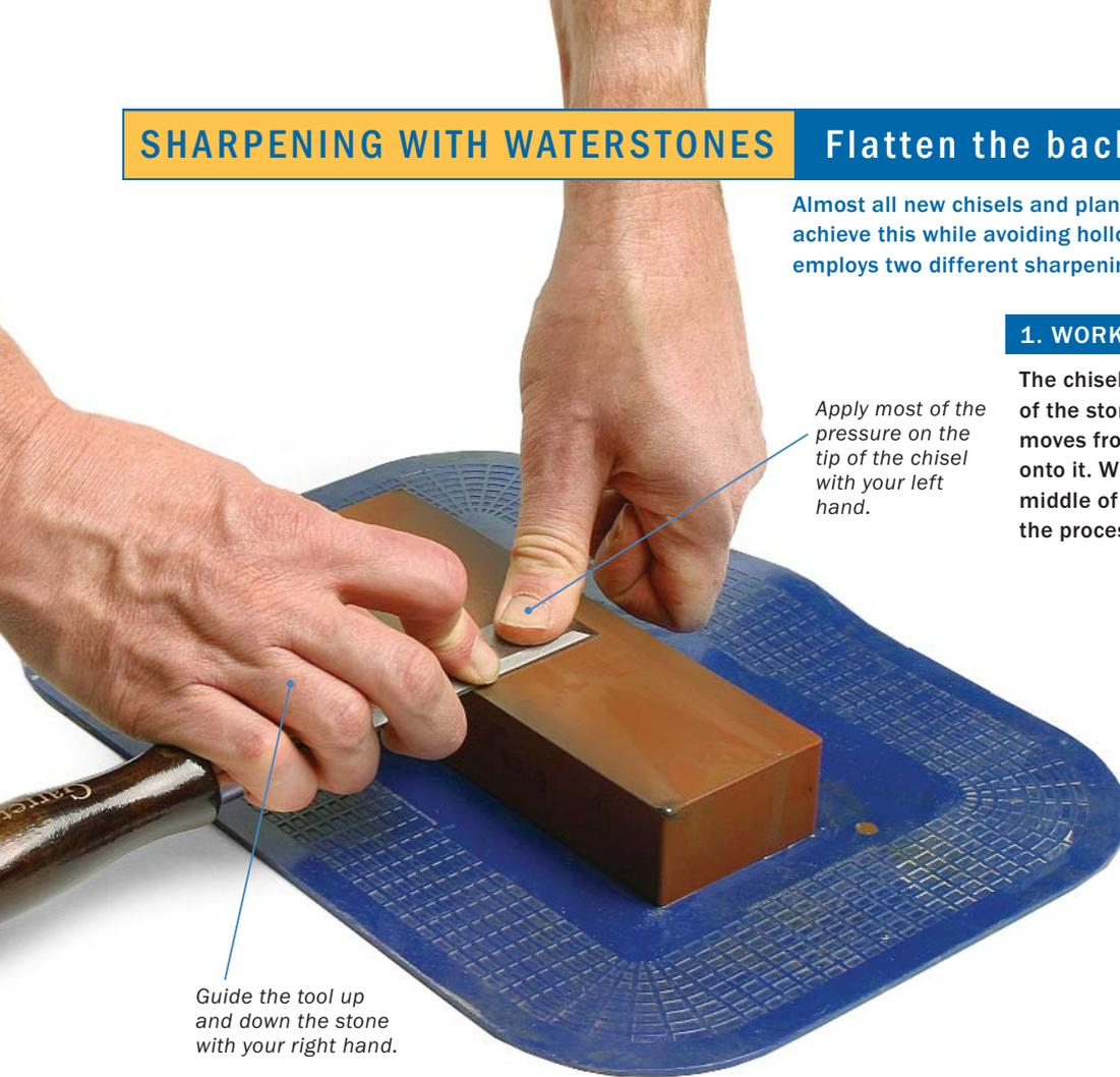
Apply most of the pressure on the tip of the chisel with your left hand.
