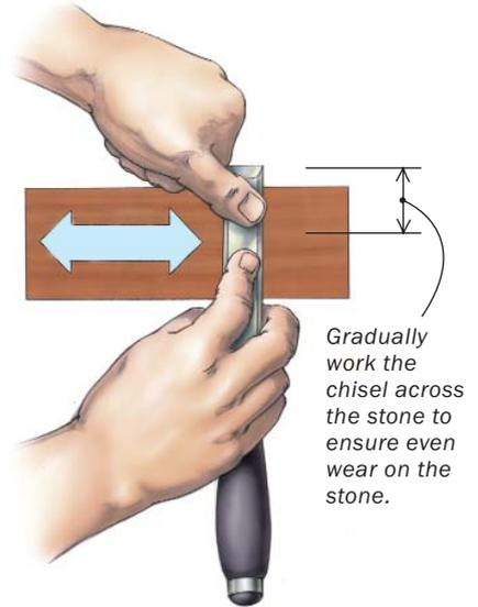
Gradually work the chisel across the stone to ensure even wear on the stone.
