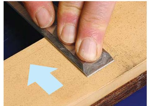
**Remove the wire edge.** Pull the back of the chisel onto the 8,000-grit stone a couple of times to roll this thin burr around, and then make a few crosswise passes to remove it.
