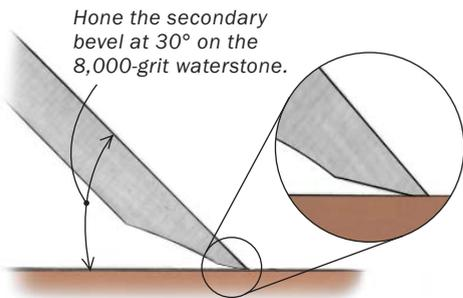
metal will be removed from this critical area. I can see no reason to polish any other part of the blade except this vital area adjacent to the tip, which forms half of the cutting edge.
