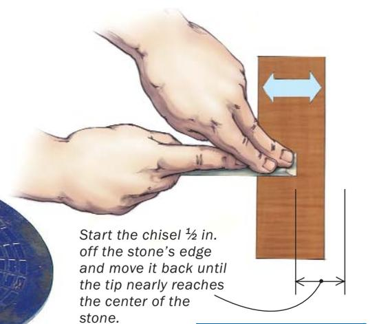
Start the chisel  $\frac{1}{2}$  in. off the stone's edge and move it back until the tip nearly reaches the center of the stone.
