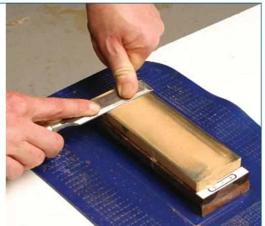
The same two types of strokes that were used on the coarser stones are used on the 8,000-grit stone. The aim is to keep the back flat while polishing the area behind the tip of the blade.
