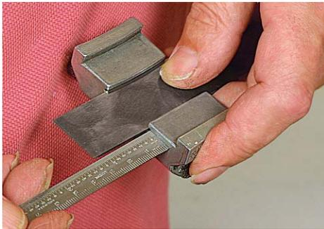
**Reset the honing guide.** To achieve the angle for the third bevel, withdraw the tip of the chisel about  $\frac{1}{8}$  in.
