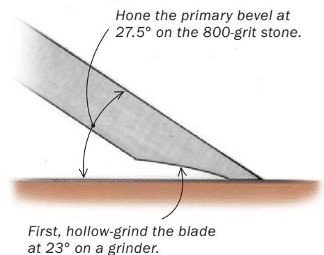
chisels and plane blades to become convex in their width. The crosswise grinding stroke is much shorter and across the stone: The chisel tip starts off the stone and moves to a point one-third to halfway across its width. Gradually work down the length of the stone and back again; then rotate the stone 180° and use the other half of the face. When this is done, flatten the stone again and repeat the first type of stroke.
