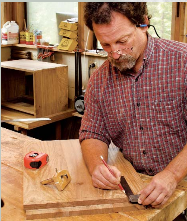
Lay out one side of the joint. Mark the cheeks with a square, but use a marking gauge to scribe the depth, setting the gauge to the thickness of the mating piece.
