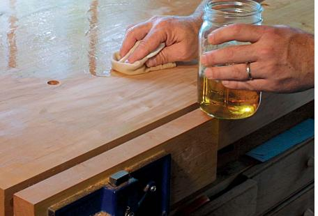
Lay it on heavy. Apply the oil-varnish mixture liberally and allow it to soak in for 10 minutes before wiping off the surplus with a clean cloth.
