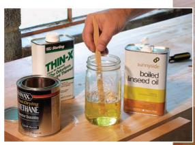
**Mix the finish.** Minick's mixture of oil, varnish, and paint thinner contains a higher proportion of resin than most Danish oils to give the bench greater protection.
