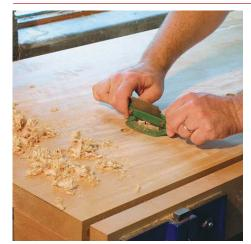
**Scrape first.** On a used bench, scrape away any dried glue before applying a new coat of the wipe-on finish.
