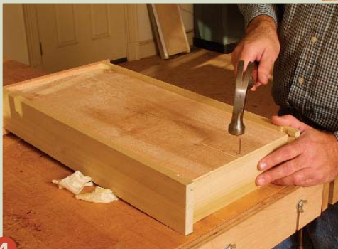
4 Nail keeps the bottom from moving when the drawer is opened.
