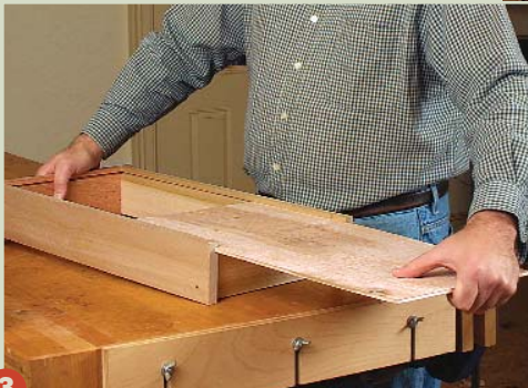
3 Plywood bottom slides in from the back.
