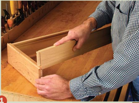
1 Drawer sides mate with dovetail slots in the drawer front.
