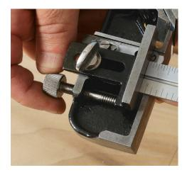
While wooden planes can employ two other styles of depth stop, Rozaieski prefers the screw stop. Typically made of brass, it's mortised into the plane body and adjusted with a thumbscrew located on top of the plane body.
