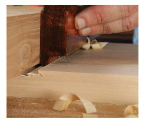
of the plane body. Another possibility is that you are tipping the plane. If you start nice and vertical but then tip the plane as your dado progresses, the front corner of the plane will rub on the wall of the dado, causing the plane to bind. Again, slow down and focus on holding the plane plumb.
