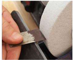
The skewed main blade should project evenly from the mouth. To verify this, color the back of the iron and place it in the plane. Scribe the iron following the sole of the plane. The scribe line will show clearly against the marker. Grind a new bevel at the proper skew angle if necessary. Begin with the blade horizontal, grinding the tip until you reach your scribe line. Then tilt the blade up to form the bevel.
