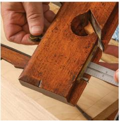
not interchangeable between planes of different widths. Each scoring blade attaches to the plane with two small machine screws that easily go missing, so check for all four.
