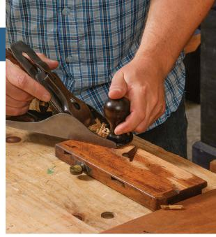
To work properly, the sides of a plane's body must be straight. If they're out more than 1mm, pass on the plane and keep looking. Anything more, and fixing the bow will negatively affect the tool. The sole should be straight and square, too. Use a very finely set bench plane to make adjustments. If the body is slightly bowed, straighten its right side for accurate reference on the batten when using the plane. Then joint the sole.
