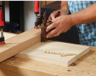
across the fibers, so you want the geometry to be right. If it isn't, grind a new bevel at the proper angle. Then, hone the edge. I find this easiest to do freehand.
