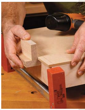
Start attaching the bottom at a front corner. Use a little alignment jig to set the overlap, and make sure the bottom is flush at the front edge. Then shoot one 1½-in. brad at that corner, and a row along the front edge.
