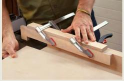
**Crosscut the rest on a big sled.** For all but the largest panels, Christiana used a crosscut sled with a 24-in. by 48-in. base. For consistent cuts on parts longer than the sled, he clamped a hook stop to the fence.
