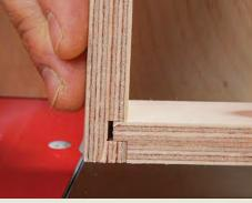
**Rabbet makes the tongue.** The next step is rabbeting the ends of the drawer sides to form a small tongue, using the same 1/4-in. dado stack, buried slightly in a sacrificial rip fence. Using test pieces, start by dialing in the cutting height (left) and the resulting tongue thickness (right), and then move the rip fence to set the length of the tongue.
