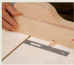
**Box-jig basics.** Cut a <sup>1</sup>/<sub>4</sub>-in. slot in an auxiliary fence and glue in a key of the same width. Sand or chisel a little taper on its top edges before gluing it in place, to encourage the workpiece dadoes to drop onto it. Then clamp the fence to your sled as shown, setting the desired distance between slots. To change the spacing, just move the fence.
