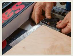
Crosscut the largest pieces against the rip fence. Find and mark a square factory corner (above), and place that against the rip fence to ensure the opposite end is cut square. Maintain pressure against the rip fence as you cut.
