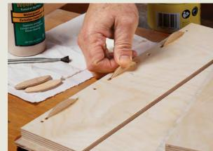
Glue goes in slots only. Put a bead in each slot, spread it with a small brush, and pop in the biscuits.
