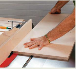
very consistent material with pretty edges. I used 3/4-in. for the cabinets, 1/2-in. for the drawer boxes, and 1/4-in. for the sliding shelves. For the cabinet backs, I went with 1/2 in. thick, to allow a strong screwed connection to the wall studs.
