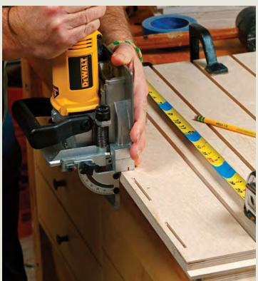
Go vertical to biscuit the sides. Space the biscuits the same way you did on the tops and bottoms, but inset the layout marks from the edge to make them visible along the bottom of the machine's base. Make sure the fence is tight to the edge as you cut slots, and support the base as shown to keep it from wobbling.
