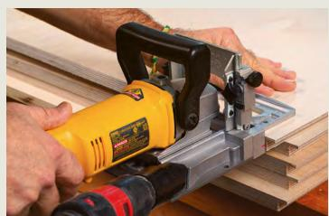
Start at the outside edges. To locate the outside slots quickly and accurately, reference the edge of the base on the edges of the workpiece. At the back edge, use the inside of the rabbet. Also, make sure the fence is resting on the outside face of each piece.
