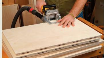
Use layout marks for the rest of the slots. Mark their locations on blue tape (far left), stuck to your measuring tape, and you'll eliminate measuring errors. Hold the tool's fence as shown (left) to keep it flat and stable as you cut.
