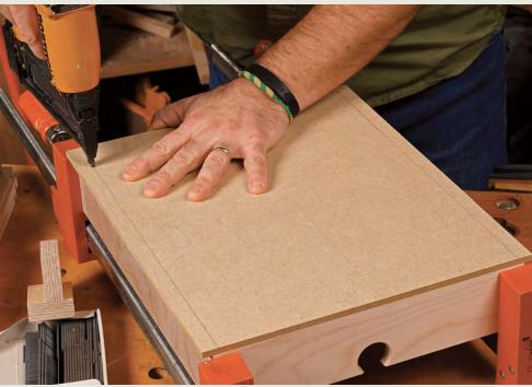
**Continue down the same side.** Use your overlap jig again near the back corner, pulling the whole box into alignment as you do, and shoot nails down the side. The layout lines help you place nails in the center of the drawer sides. To prevent brads from curling sideways and popping out, keep the gun parallel to the pieces you're nailing into. Once the front edge and one side are aligned and attached, shoot nails into the other edges.
