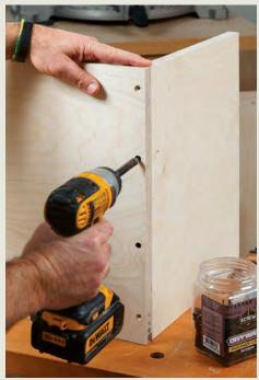
One joint at a time. Make sure the front edges are flush as you drive screws.
