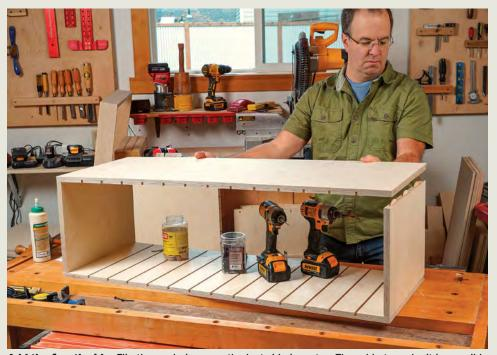
Add the fourth side. Flip the workpieces so the last side is on top. The rabbets make it impossible to reverse the pieces and misalign the rows of dadoes.
