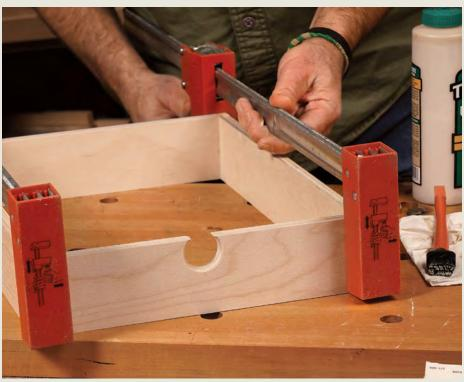
**Clamp them right-side up.** Parallel-jaw clamps work well here. Make sure the top edges of the box are flush and the clamps don't extend past the bottom edge.
