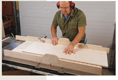
Back edges get rabbets. Set up a wider dado stack and bury it partially in a sacrificial rip fence. To be sure you rabbet the right edges, start by matching up slots in mating sides and marking their back edges. Cut a test piece to be sure the ½-in. plywood back will end up flush at the back edge.
