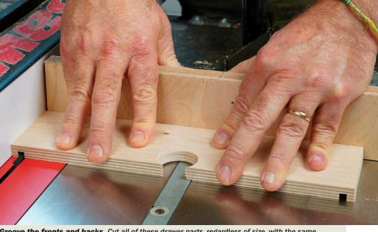
**Groove the fronts and backs.** Cut all of these drawer parts, regardless of size, with the same setup. The miter gauge guides the workpieces—with a sacrificial fence preventing tearout—and the rip fence acts as a stop.
