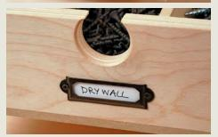
The tongue-and-grooved drawers have a nailed-on MDF bottom that slides into slots in the cabinet sides. Other details include drilled finger pulls, label holders, and drawer dividers fixed in place with hot glue.
