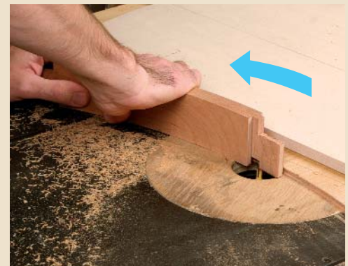
Curved fence to rout a curved groove. After cutting and smoothing the curves in the rails, use the curve template to make a curved fence for the router table. Keep the workpiece steady on the table as you slide it along the fence.
