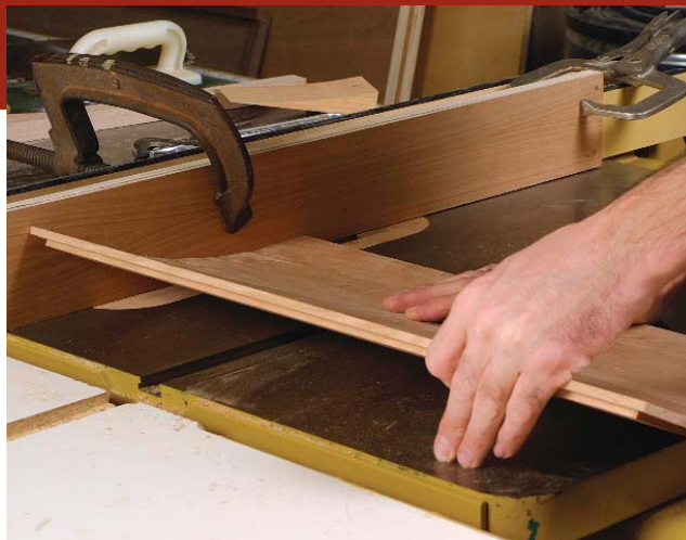
Rabbet the curved edge. Use a good dado set and keep the panel in contact with the table at the cutting point. The rabbet also may be cut on the router table.
