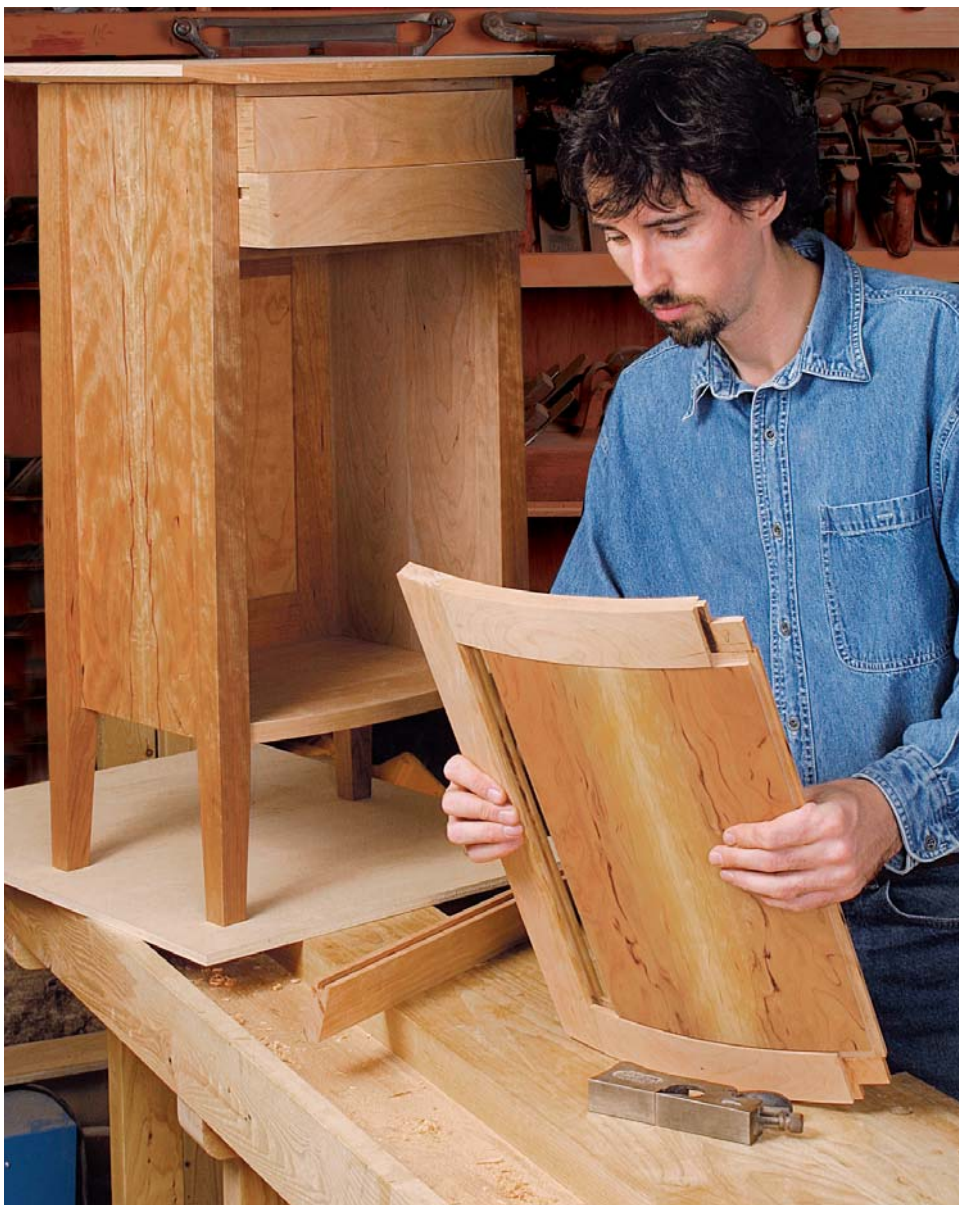
Prefinish the panel and dry-fit the door. Use a shoulder plane to fine-tune the joinery.
