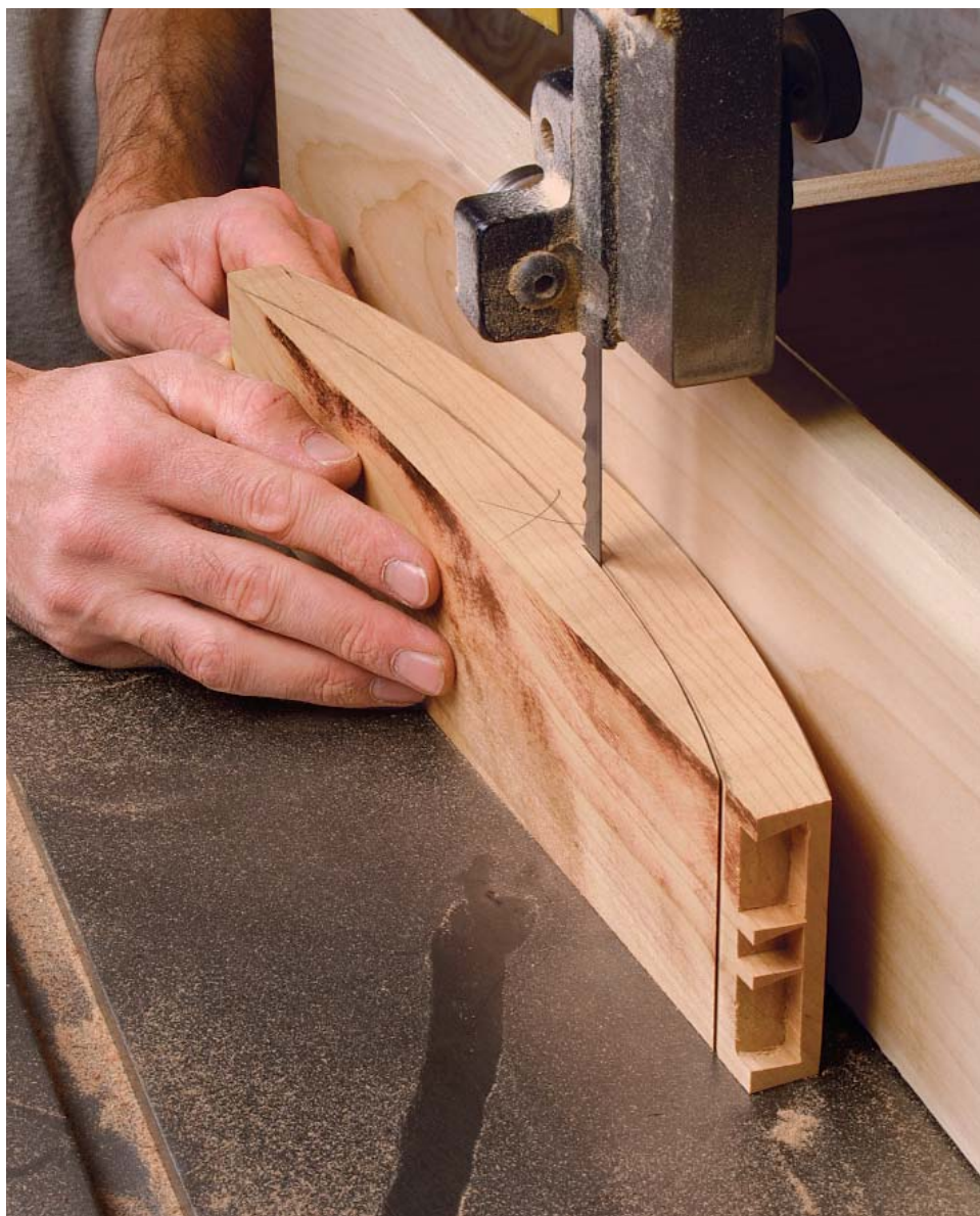
An easy way to cut the inside curve. Lay out the desired curve. Then ride the rip fence as shown to follow that curve, creating a consistent thickness. Use the offcut as a sanding block.
