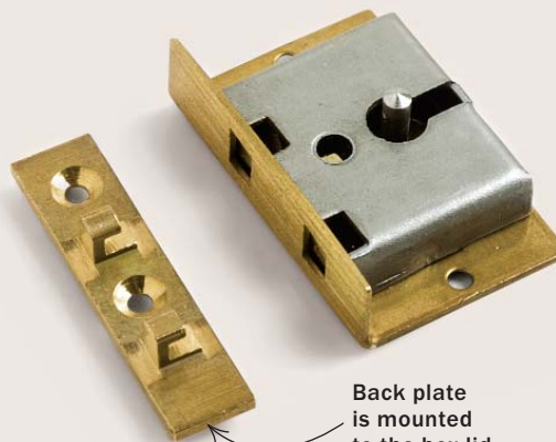
Locksets for small boxes are no different from those used on blanket chests. The lockset is mortised into the box, and two hooks in the mating back plate in the lid seat themselves in the lockset.
