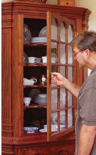
The lockset installed on this door is typical of those found on most 18th-century doors and drawers. It is mortised into the back of the door. A mortise in the opposing door or case captures the bolt.
