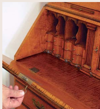
When a slant-front desk lid closes, the rabbet on its edge is angled to meet the case piece. The angle of the desk lid must match the angle on the back plate of the lockset.
