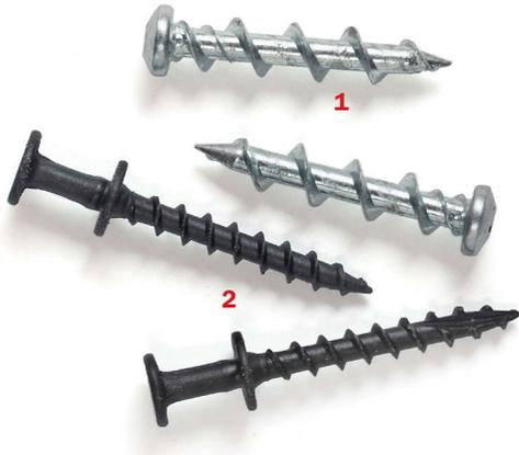
For some light-duty applications, like smaller picture frames or a light display shelf, you can actually use coarse-threaded screws designed to be driven into drywall without an anchor or a pilot hole. They're rated to hold as much weight as plastic sleeve anchors, and they
