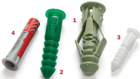
The Cobra Triple Grip (1), intended for all wall types, is rated for 46–61 lb. in drywall, 200–225 lb. in masonry; Everbilt Ribbed Plastic Anchors (2 and 3), which come in kits of assorted sizes, are rated for 20–25 lb. in drywall, 155–435 lb. in concrete; Duo Power plastic anchors (4) elbow open and are rated for 45 lb.
