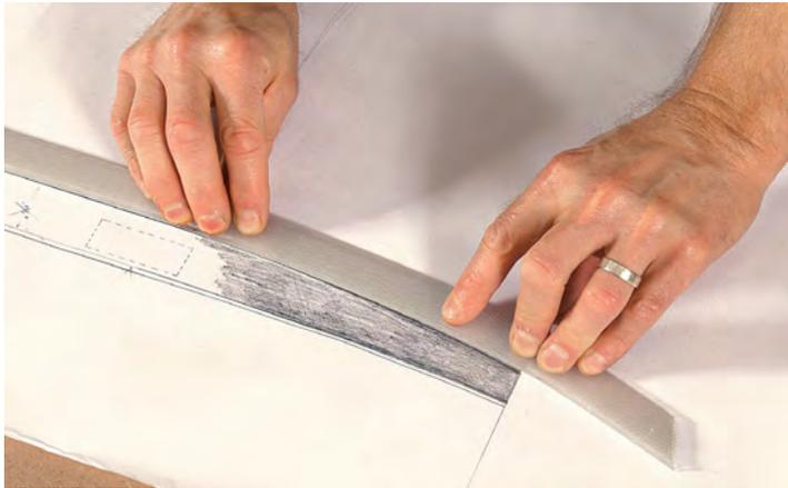
**An adjustable curve allows for more versatility.** This tool is a series of thin plastic strips that are keyed to each other and fixed on one end to allow the tool to bend to fairly intricate shapes. Korsak lays down a few short pieces of blue tape across the plastic strips to secure the shape when transferring it between a drawing and a furniture part.
