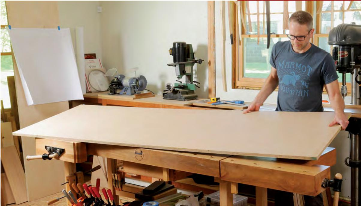
Instead of creating a dedicated drafting space in his midsize shop, Korsak pulls out a sheet of MDF as an on-demand drafting board when needed. Its smooth surface is ideal, and it can be cut to appropriate size and stowed away easily.
