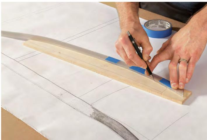
ranging from drawer pulls to tabletops. For more complex curves, I rely on French curves, an adjustable curve, and a pair of drawing bows, one for symmetrical curves and another for asymmetrical. Because I often use just a section of these tools, I mark the area with blue tape.
