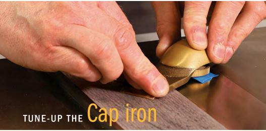
Use sandpaper to flatten the underside of the cap iron where it will contact the blade. With a file and diamond hones, smooth and polish the cap iron's rounded front edge to ease the flow of shavings over it.
