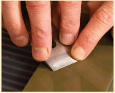
Cambering the blade slightly keeps the corners from digging into the wood and leaving tracks. To produce the camber, hone the blade as usual, then take a few strokes while focusing pressure first on one corner, then the other.
