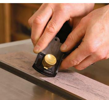
Rounding over any sharp edges around the perimeter of the sole makes the plane friendlier to handle and prevents scratches to the workpiece.
