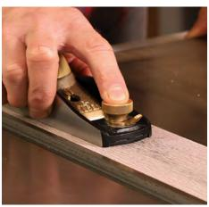
Rubbing the plane over 320-grit sandpaper adhered to a flat surface makes quick work of minor imperfections. To simulate the stresses on the plane when in use, be sure to have the blade in place (though retracted) and the cap iron on while flattening.
