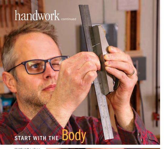
Holding the plane up to a light source, check with a straightedge to see if the sole is flat. Check down the middle, at the sides, and on the diagonals as well. If you see any glint of light, mark the location.
