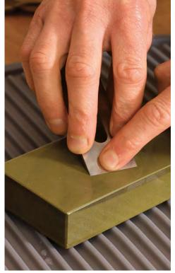
After hollow-grinding the bevel, Korsak uses a waterstone to flatten the back of the blade. Then he hones the bevel.
