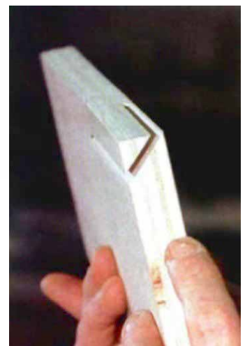
How much to cut. The miter should not reduce the width of the workpiece, which is cut to finished dimensions first.
