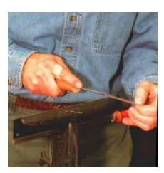
Sharpening a backsaw is a skill. A single pass will sharpen the teeth on this dovetail saw. Each stroke has to be even to keep the teeth uniform.
