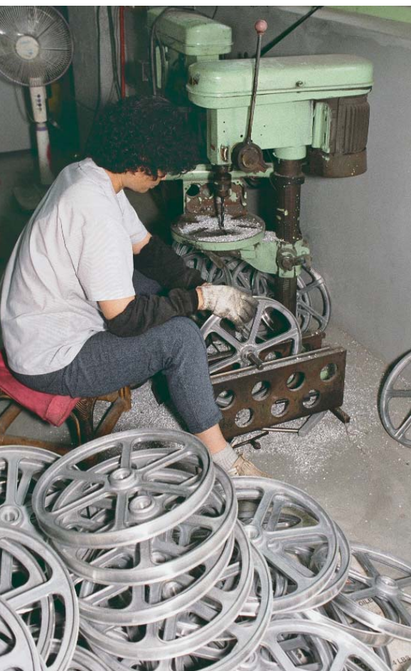
Two ways to balance a wheel— A worker at the Grizzly factory (above) uses a modern electronic tool to balance a bandsaw wheel. The woman (left) at the Shih Hsin factory uses a mechanical method to perform the same task. Both workers use a drill press to remove small amounts of material when one section of the wheel is heavier.
