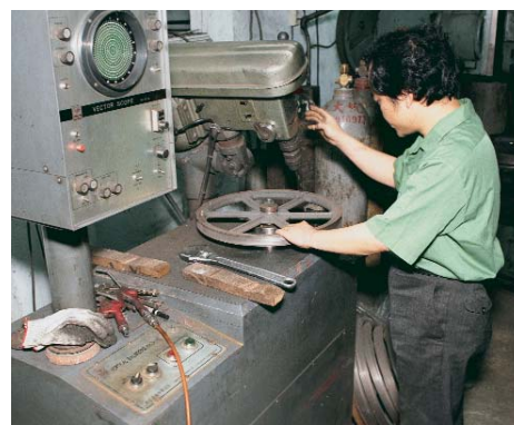
Two ways to balance a wheel— A worker at the Grizzly factory (above) uses a modern electronic tool to balance a bandsaw wheel. The woman (left) at the Shih Hsin factory uses a mechanical method to perform the same task. Both workers use a drill press to remove small amounts of material when one section of the wheel is heavier.
