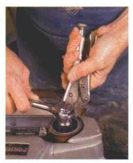
**Hold still.** An old leather belt and a pair of Vise-Grips hold the rubber drive wheel as the author backs off the axle nut (above). Tire-traction compound improves the grip (right).
