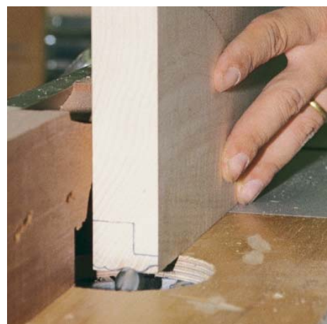
Shape the frame. Start with wide stock. When using multiple router bits, sketch the molding profile before beginning.
