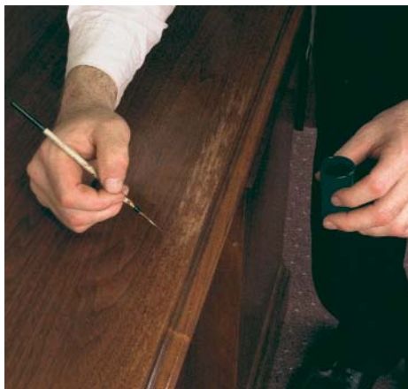
No stripping required. Working with alcohol-soluble dyes and a fine brush, the author makes repairs to this walnut desk that will be virtually undetectable.
