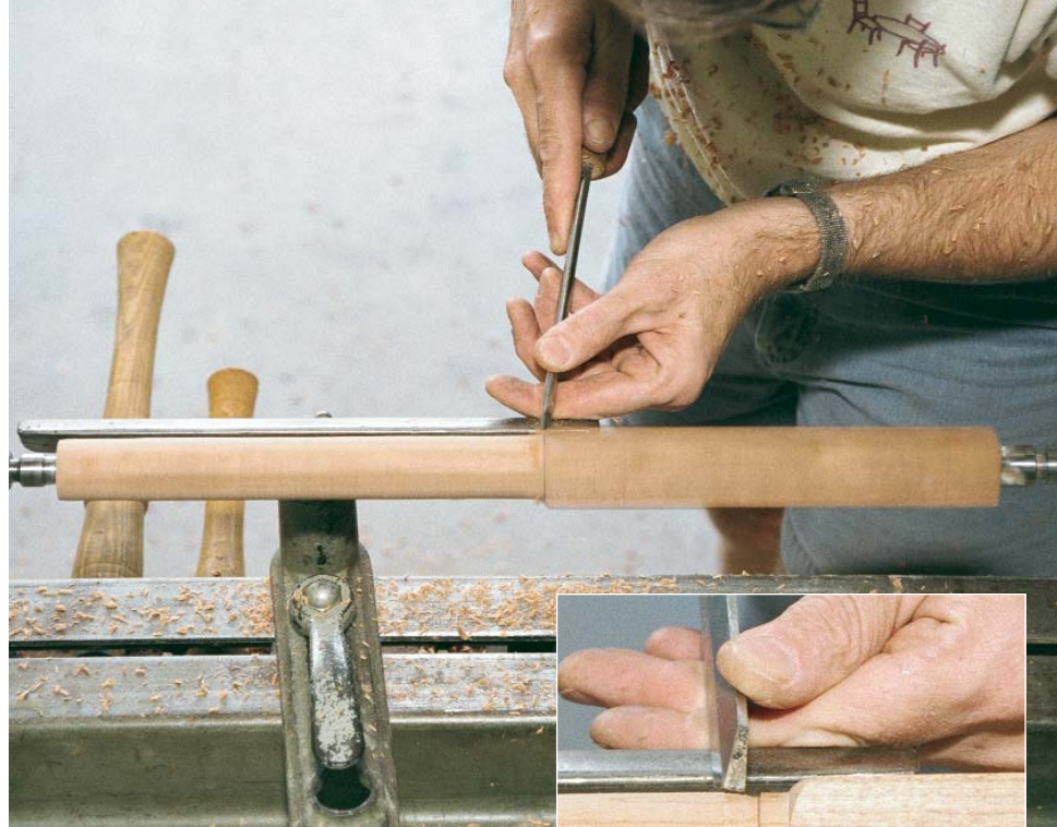
The tough part is the transition. The point where the leg turns from square to round is easy to ruin. An initial cut with a skew (above) can prevent chipping. A parting tool (right) helps form the collar.
