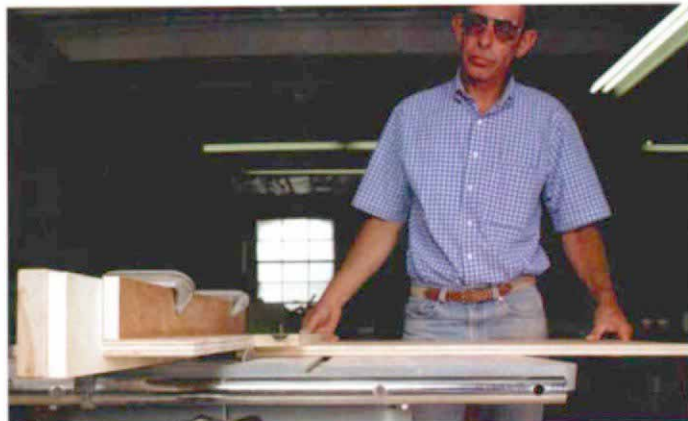
2. Run the workpiece through the saw, keeping even pressure on the straightedge against the jig.
