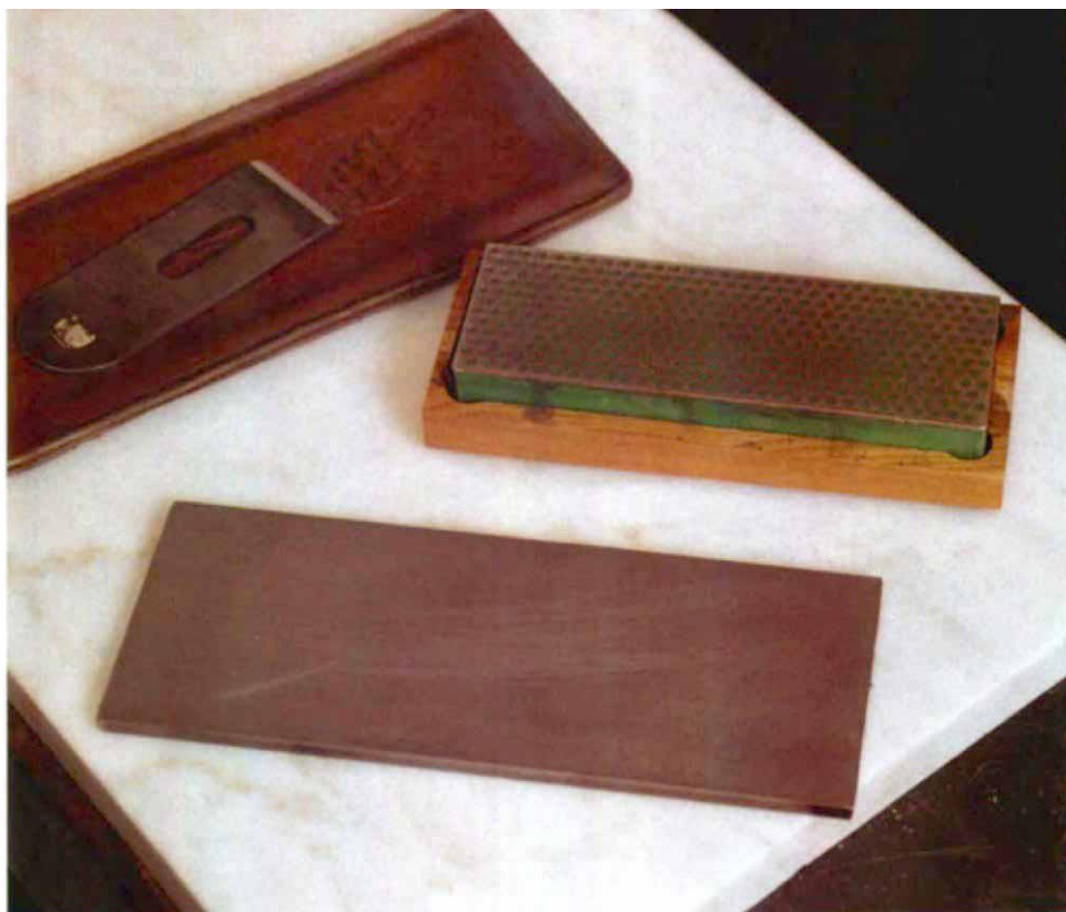
Two types of diamond plates—The DMT plate, top, has a perforated surface. The surface of the Eze-Lap is solid. Both can handle high-carbon and high-speed steel tools.
