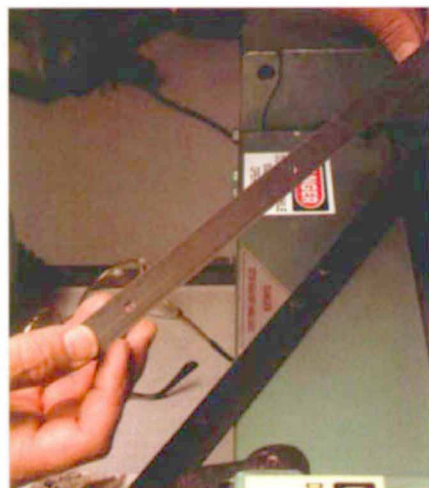
Esta disposable knives —Double-edged knives fit into a holder that rests on height-adjustment screws. Same gib and gib screw setup.
