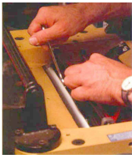
Typical cutterhead —Knives rest on springs and are held in place by gibs and gib screws.
