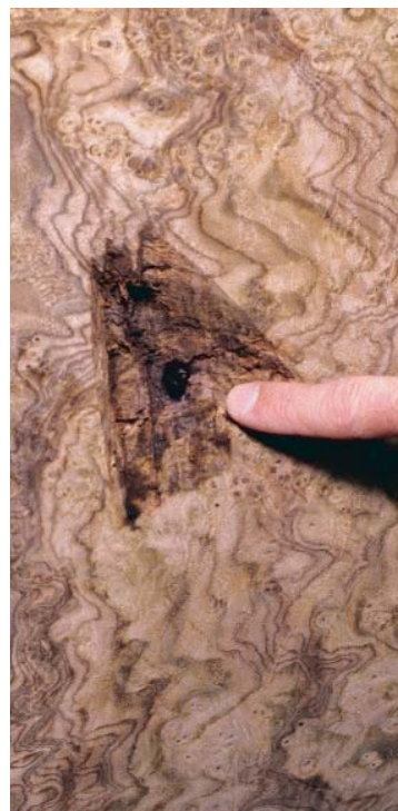
The enemy is metal. A worker points to a nail found in a walnut burl. The lathe operator periodically stopped the machine and chopped around the nail with an ax to remove it bit by bit and prevent damage to the knife.
