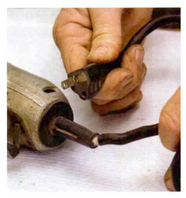
Cord breaks often occur near strain reliever. The plug on this cord is missing the grounding prong and needs to be replaced.
