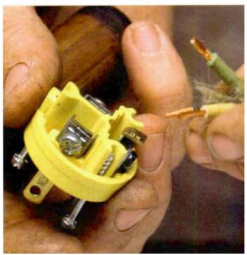
If you think the wire break is located near the plug, cut the cord there, and perform another continuity check on the bare wires between the switch and the cut end of the cord. If you get a zero reading, celebrate by installing a new aftermarket plug, available in any hardware store (see the bottom photo). Be sure to use a three-prong plug if that's what the tool came with. A tool with a metal housing must be grounded to avoid a serious shock hazard. Double-insulated
