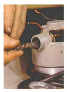
With cap removed, brush pops out. Spring-loaded brushes should come out of their guide channels easily once the end caps are out of the way.
