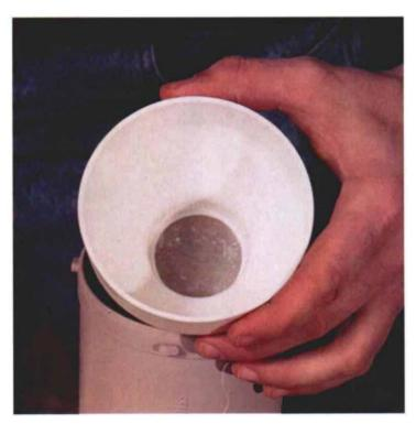
Get the lumps out. Waterborne finishes have a high solids content, so it's important to strain the material before spraying.
