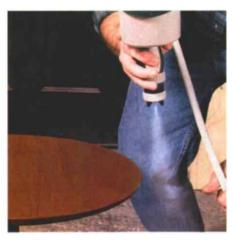
Begin spraying before you reach the workpiece. Hold the gun 4 in. to 6 in. away from the workpiece, and spray at a speed that makes the surface wet and shiny but not runny.
