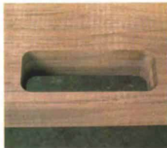
First pass with pattern bit
